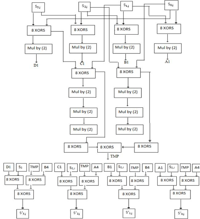
Fig. 4. Inverse mix columns operation
