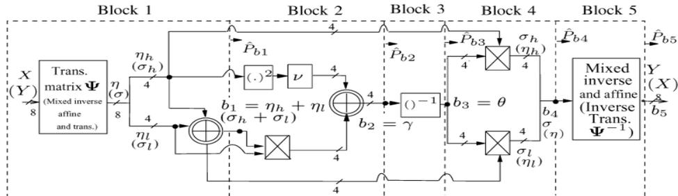
Fig. 1. The S-box (the inverse S-box) using composite fields and polynomial basis and their fault detection blocks.
