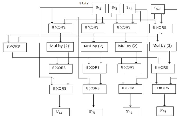
Fig. 3. Forward mix columns operation
