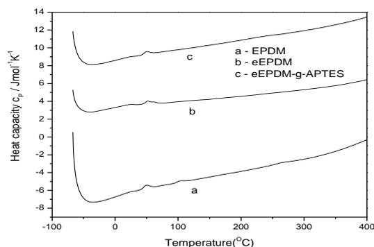
Fig. 7. DSC curves of (a) EPDM (b) eEPDM (c) eEPDM-g-APTES
