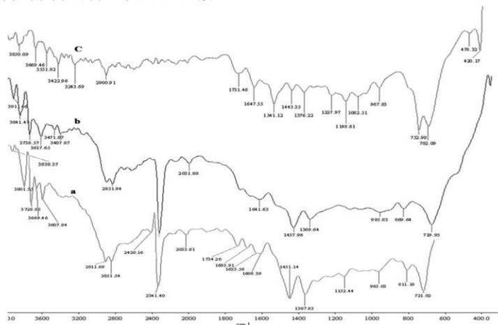
Fig. 1 FTIR spectra of (a) EPDM (b) eEPDM and (c) eEPDM-g-APTES
