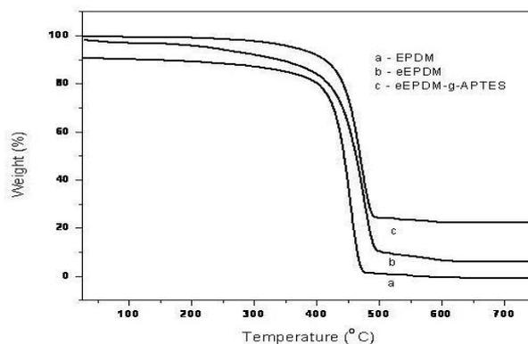
Fig. 6. TGA curves of (a) EPDM (b) eEPDM (c) eEPDM-g-APTES
