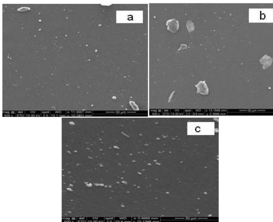
Fig. 8. SEM photographs of (a) EPDM (b) eEPDM (c) eEPDM-g-APTES
