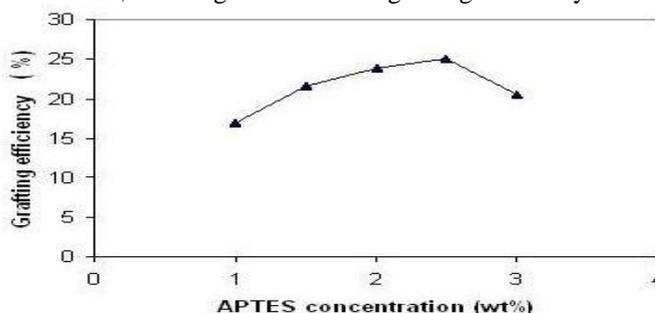
Fig.3. Plot of grafting efficiency against APTES concentration (reaction temperature, 80°C; reaction time, 4 h).
