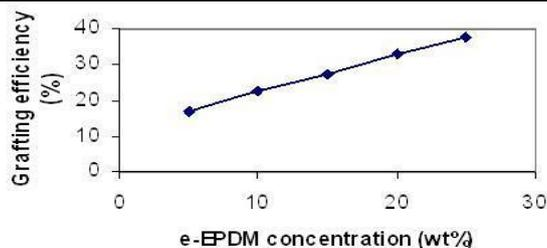
Fig.2. Plot of grafting efficiency against eEPDM concentration (APTES, 2.5 wt%; reaction temperature, 80°C; reaction time, 4 h).
