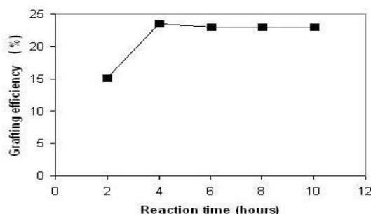
Fig.4. Plot of grafting efficiency against reaction time ((APTES, 2.5 wt%; reaction temperature, 80°C).
