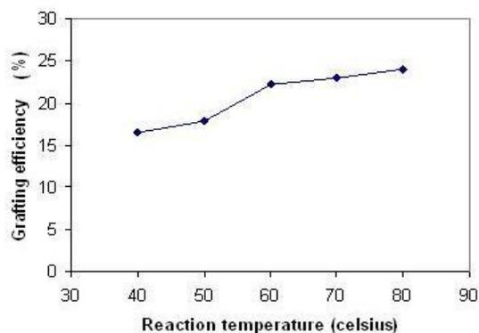
Fig.5. Plot of grafting efficiency against reaction temperature ((APTES, 2.5 wt%; reaction time, 4 h).
