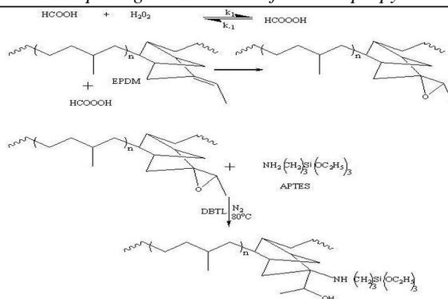
Scheme 1 Schematic representation of grafting between eEPDM and APTES
