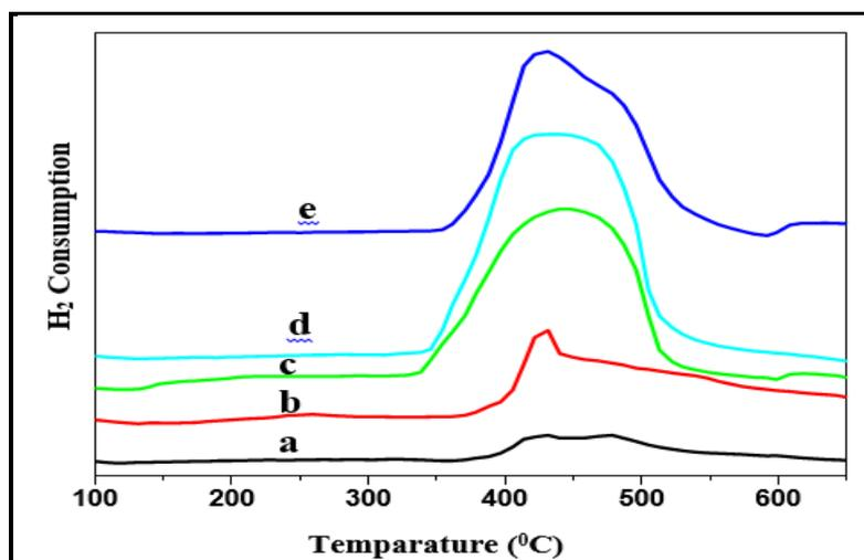
Fig.4 TPR profiles of (a) 5Ni-RHSiO<sub>2</sub> (b) 10Ni-RHSiO<sub>2</sub> (c) 20Ni-RHSiO<sub>2</sub> (d) 30Ni-RHSiO<sub>2</sub> (e) 40Ni-RHSiO<sub>2</sub>
