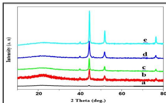
**Fig.1 XRD patterns of reduced catalysts (a) 5Ni-RHSiO<sub>2</sub> (b) 10Ni-RHSiO<sub>2</sub> (c) 20Ni-RHSiO<sub>2</sub> (d) 30Ni-RHSiO<sub>2</sub> (e) 40Ni-RHSiO<sub>2</sub>**
