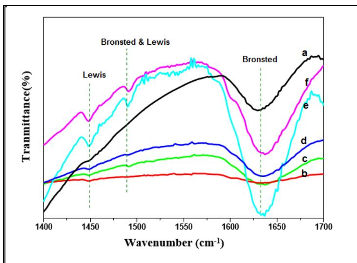
Fig.3 Pyridine adsorbed FT-IR patterns (a) RHSiO<sub>2</sub> (b) 5Ni-RHSiO<sub>2</sub> (c) 10Ni-RHSiO<sub>2</sub> (d) 20Ni-RHSiO<sub>2</sub> (e) 30Ni-RHSiO<sub>2</sub> (f) 40Ni-RHSiO<sub>2</sub>
