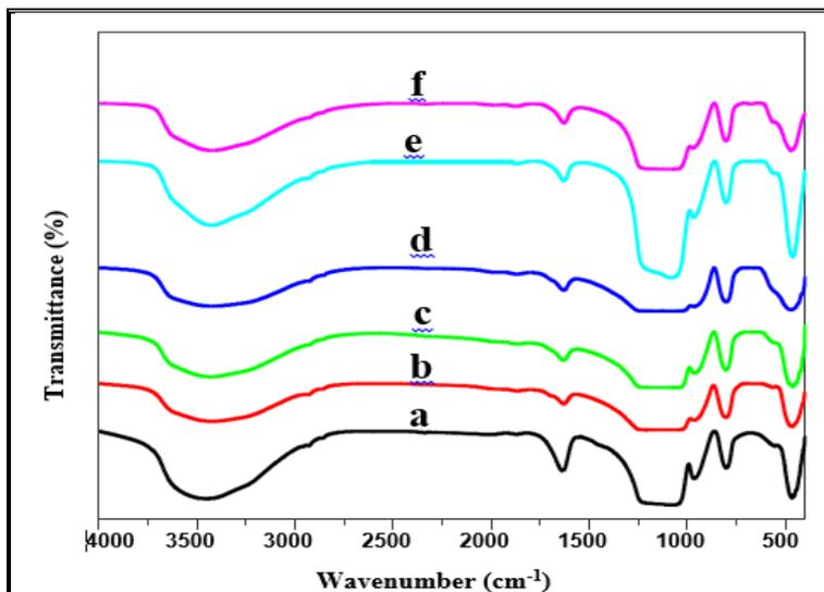
Fig.2 FT-IR patterns of (a) RHSiO<sub>2</sub> (b) 5Ni-RHSiO<sub>2</sub> (c) 10Ni-RHSiO<sub>2</sub> (d) 20Ni-RHSiO<sub>2</sub> (e) 30Ni-RHSiO<sub>2</sub> (f) 40Ni-RHSiO<sub>2</sub>
