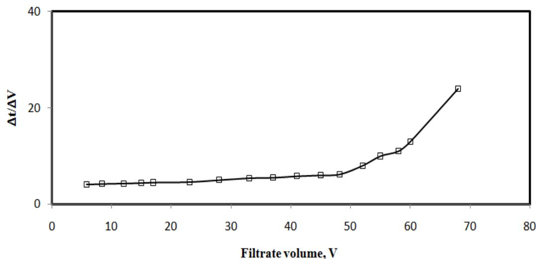
Fig. 7 Filterability Characteristics of sludge
