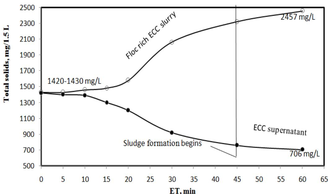
Fig. 5 Total solids removal as a function of electrolysis time
