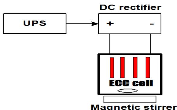
**Fig. 1** Laboratory bench scale ECC setup
