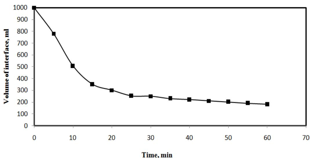
Fig. 6 Settling characteristics for Fe electrodes
