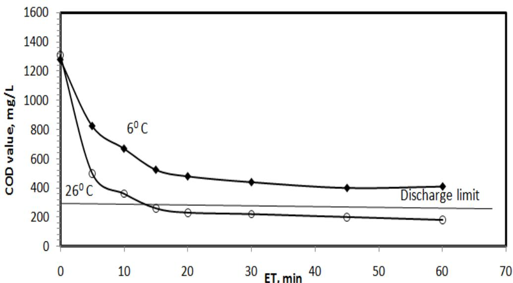
**Fig. 3** COD degradation curves as a function of electrolysis time at initial wastewater temperature of  $6^\circ\text{C}$  and  $26^\circ\text{C}$
