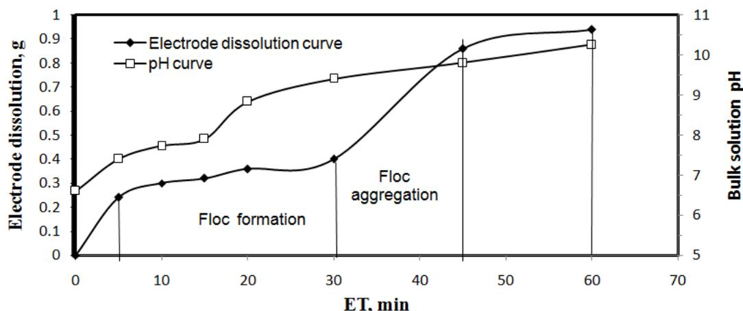
Fig. 8 Electrode dissolution and bulk solution pH as a function of ET
