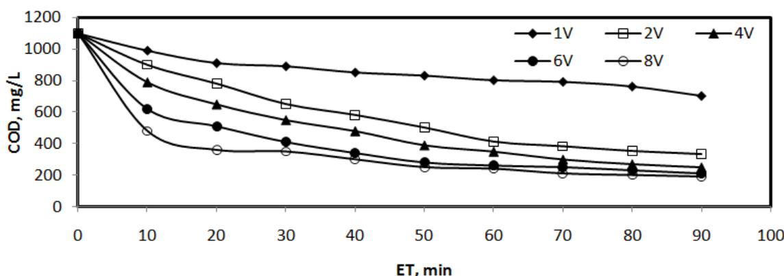
Fig. 2 COD degradation as a function of electrolysis time at different applied voltage using two Fe electrodes configuration
