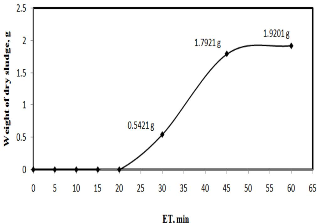
Fig. 4 Effect of electrolysis time on sludge floc formation
