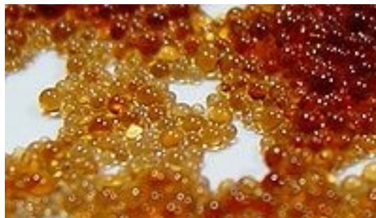
Fig.2.1. Gelular Ion exchange Resin bed
