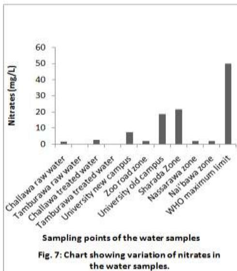
Fig. 7: Chart showing variation of nitrates in the water samples.
