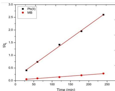
**Fig. 13. Pseudo-second-order kinetic plots for adsorption of Pb(II) ion and MB onto PCFR**
