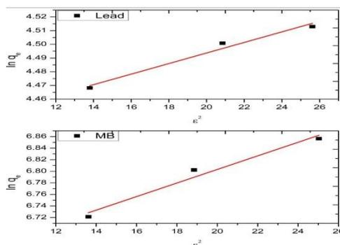
Fig.12. D-R isotherm plots for the adsorption of Pb(II) and MB onto PCFR
