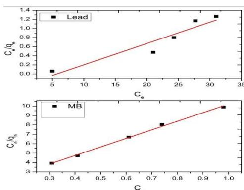
**Fig.11. Langmuir isotherm plots for the adsorption of Pb(II) and MB onto PCFR**
