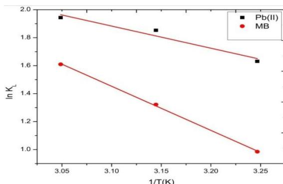
**Fig. 15. van't Hoff plots of  $\ln K_L$  versus  $1/T$  for the adsorption of Pb(II) ion and MB onto PCFR**
