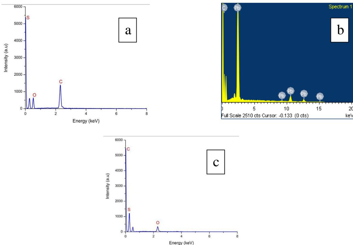
**Fig. 6. Energy dispersive spectra of (a) PCFR (b) PCFR-Pb(II) (c) PCFR-MB**
