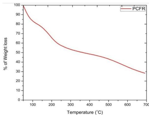
**Fig. 7. TGA curve of PCFR**
