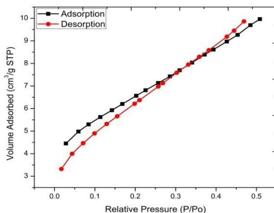
**Fig. 2. Adsorption-desorption isotherms of nitrogen at 77 K on PCFR**
