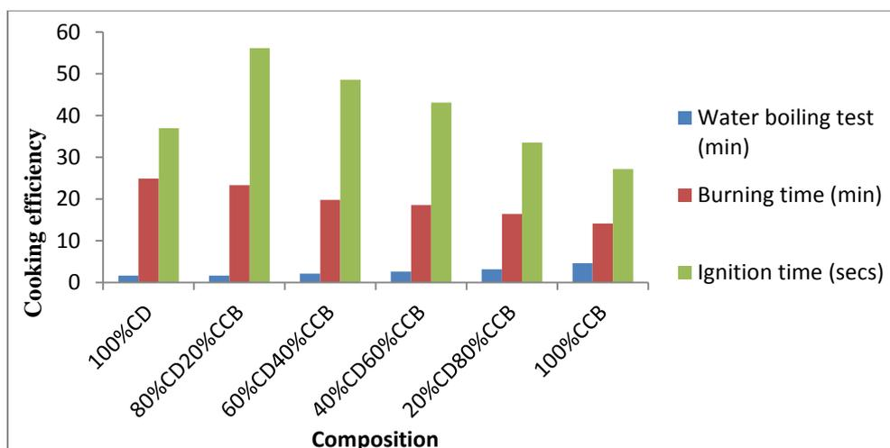
Fig. 4. Plot of cooking efficiency (water boiling test, burning rate and ignition time) of the respective briquettes produced.
