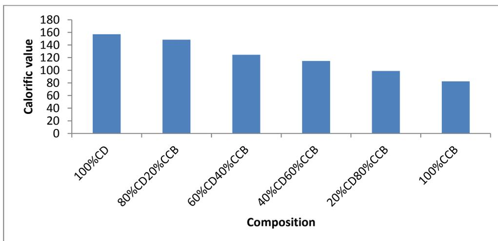
Fig. 3. Plot of the calorific values (KJ/kg) of the briquettes.
