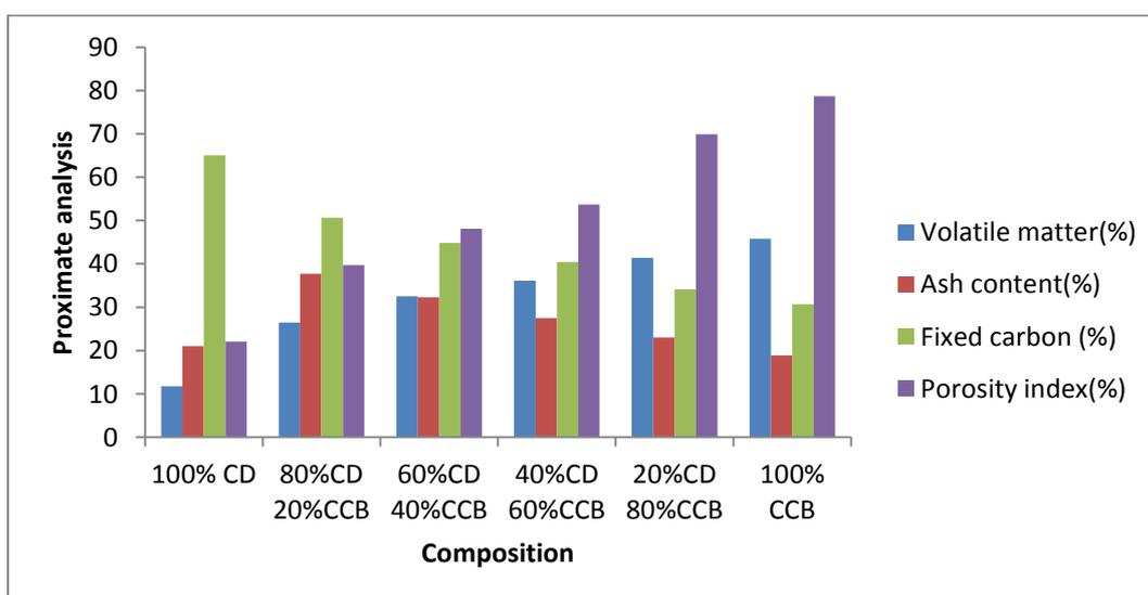
Fig 2. Plot of porosity index, fixed carbon, ash content and volatile matter of respective briquettes.
