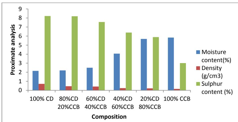
Fig 1. Plot of sulphur content, density and moisture content of the respective briquettes.
