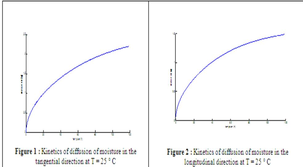
Figure 1 : Kinetics of diffusion of moisture in the tangential direction at T = 25 °C
