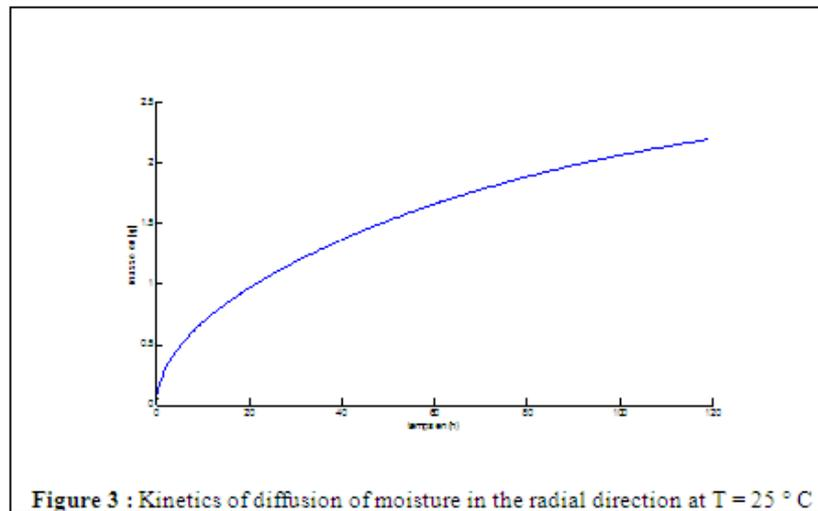
Figure 3 : Kinetics of diffusion of moisture in the radial direction at T = 25 °C
