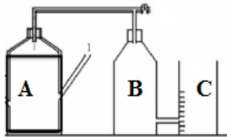
**Figure 1:** Water displacement set-up for biogas production
