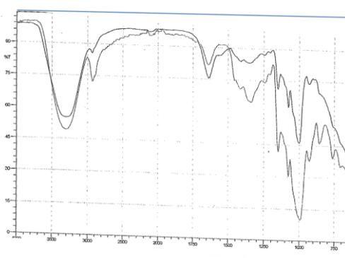
Fig.7 FTIR of starch and starch-chitosan blend
