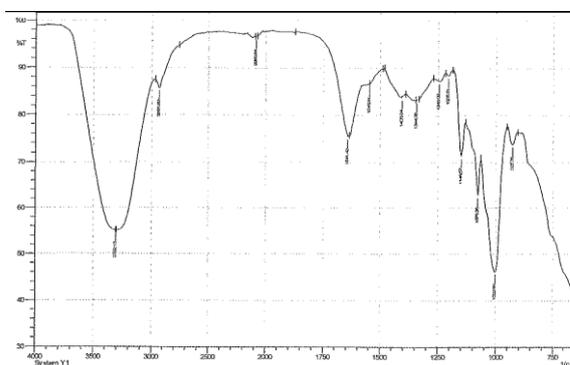
Fig.6 FTIR of starch and chitosan blend
