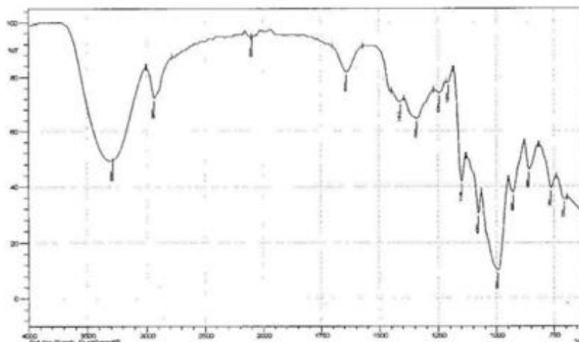
Fig.5 FTIR of soluble starch
