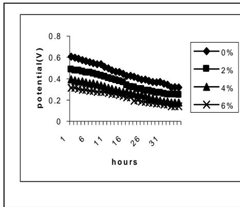
Fig 5: Open circuit potential test in 0.35 % sodium chlorides solution
