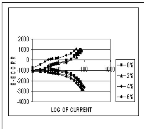
Fig 7: Potentiostat test in 0.035 % sodium chlorides solution
