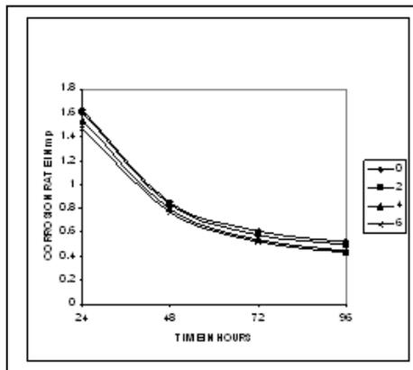
Fig.1: Weight loss corrosion in 0.035% Sodium chloride solution
