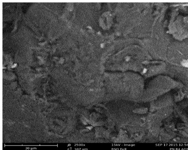
Fig. 1: SEM micrograph of PNSBP powder surface at magnification 2500×
