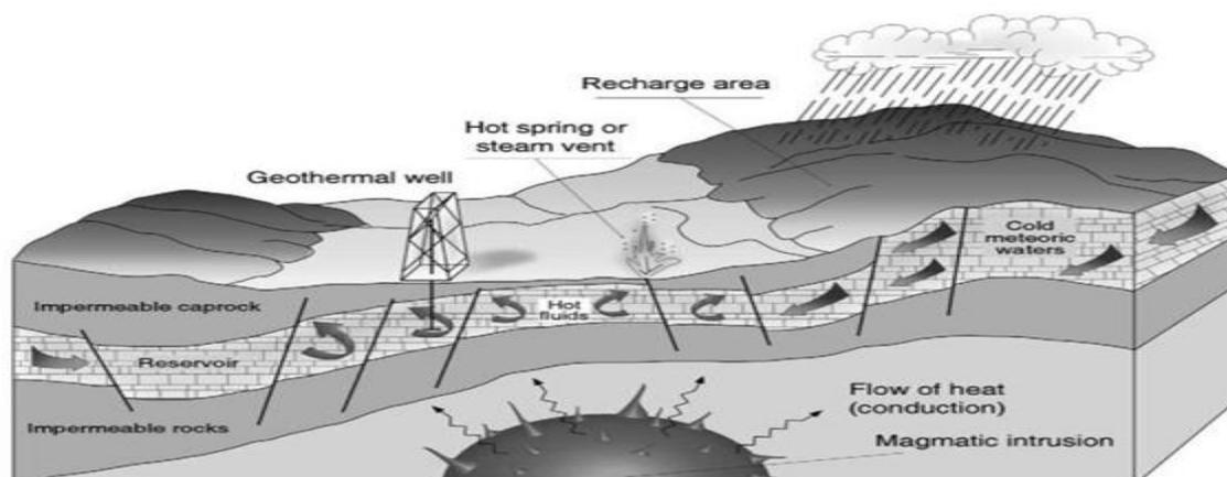
**Figure 1.1A geothermal steam field with its elements: recharge area, impermeable cover, reservoir and heat source.(Enrico Barbier 2002**
