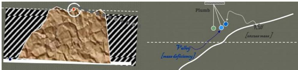
Both topographic features affect the gravity measurement in the same sense, i.e., reducing the readings due to upward attraction by the excess mass of hills or mass deficiency (less attraction), due to valleys. Terrain corrections are, therefore, always **positive**. One method of carrying out terrain correction is to divide up the area around a station into sectors bounded by concentric circles of radii drawn at suitable angular intervals. For such arrangement the correction term is given as;
