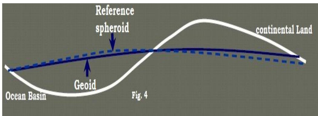
Neither the mathematical surface (reference spheroid) or the geodetic surface (geoid) consider the lateral variations in density. When these occur close to the surface, they are the object of gravity prospecting, in exploration geophysics.
