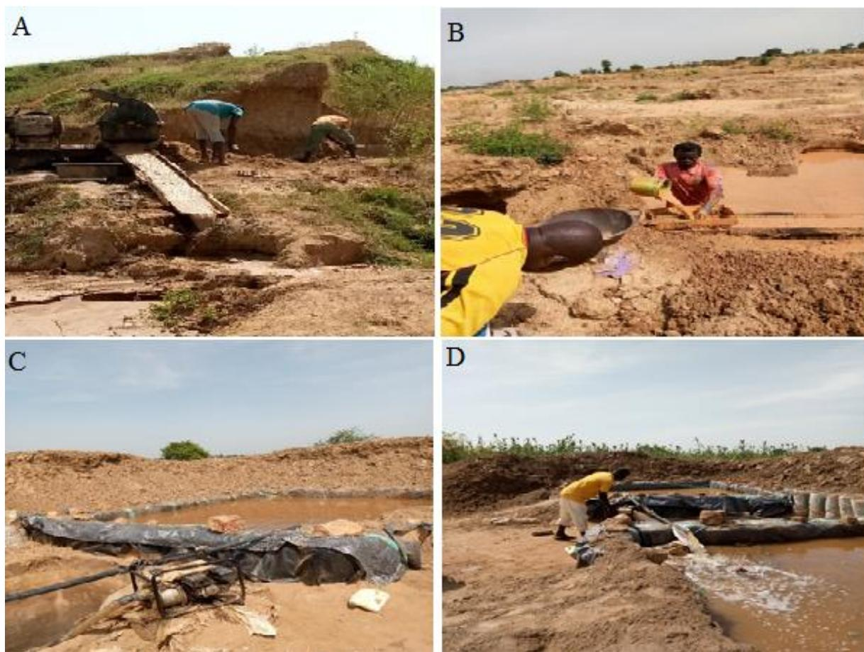
Plate V, A,B,C,D: The milling and washing of mineralized quartz vein/laterites and sedimentation in floatation tank to recover gold in the study area (11° 22' 13.7". 008° 56' 17.0").
