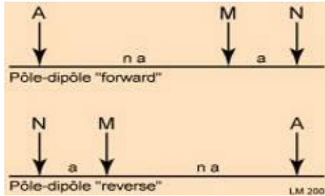
Figure 3: "Forward" and "reverse" acquisition for pole-dipole configuration
