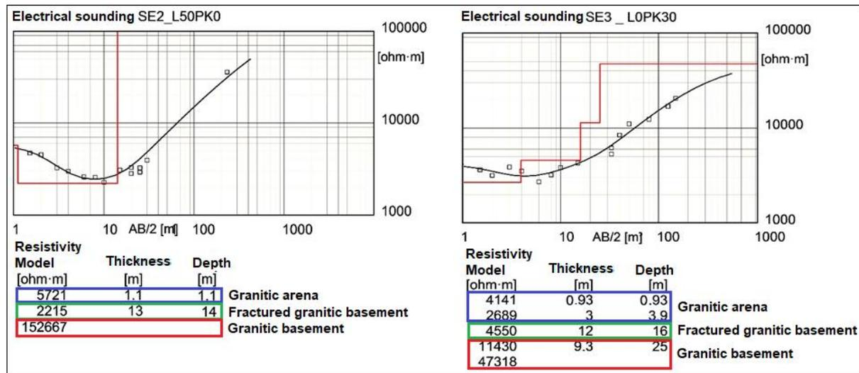
Figure 9: Sounding curves type H.
