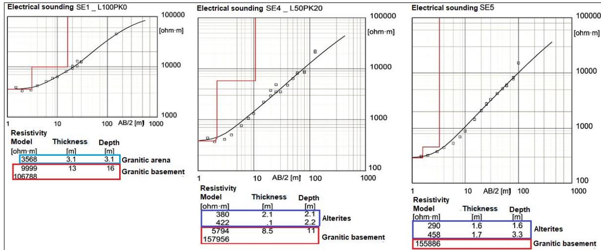
Figure 8: Sounding curves type CH1.
