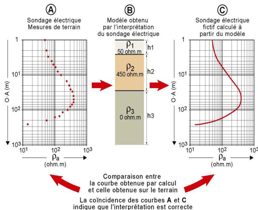
**Figure 2:** Electrical sounding curve inversion techniques [5].
