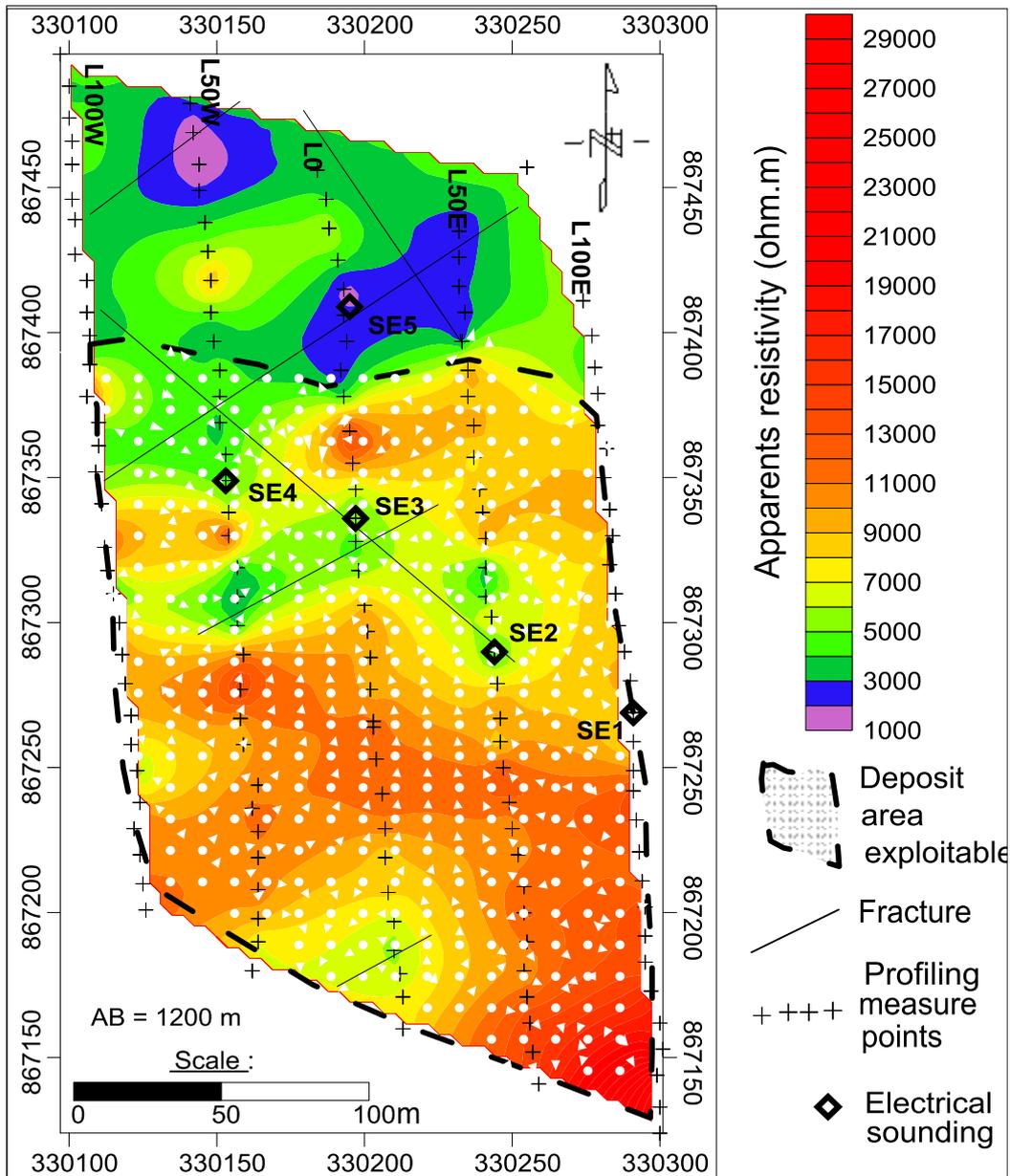
**Figure 7:** Apparent Resistivity Map of the Gbamakro Granite Deposit.
