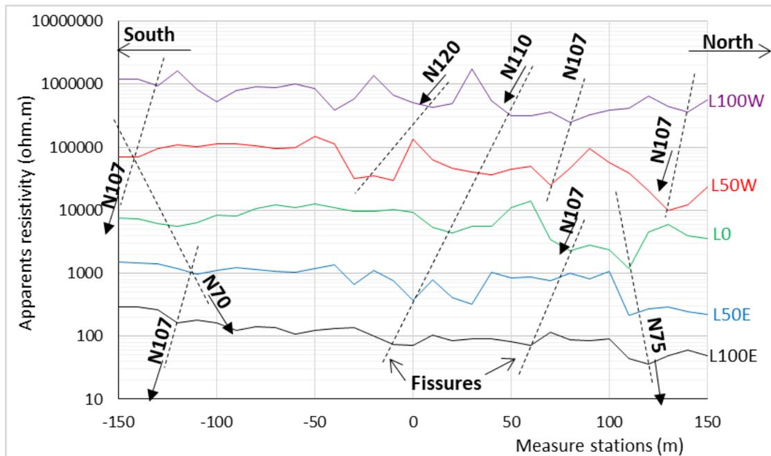
Figure 6: Resistivity profiles of the Gbamakro granite deposit
