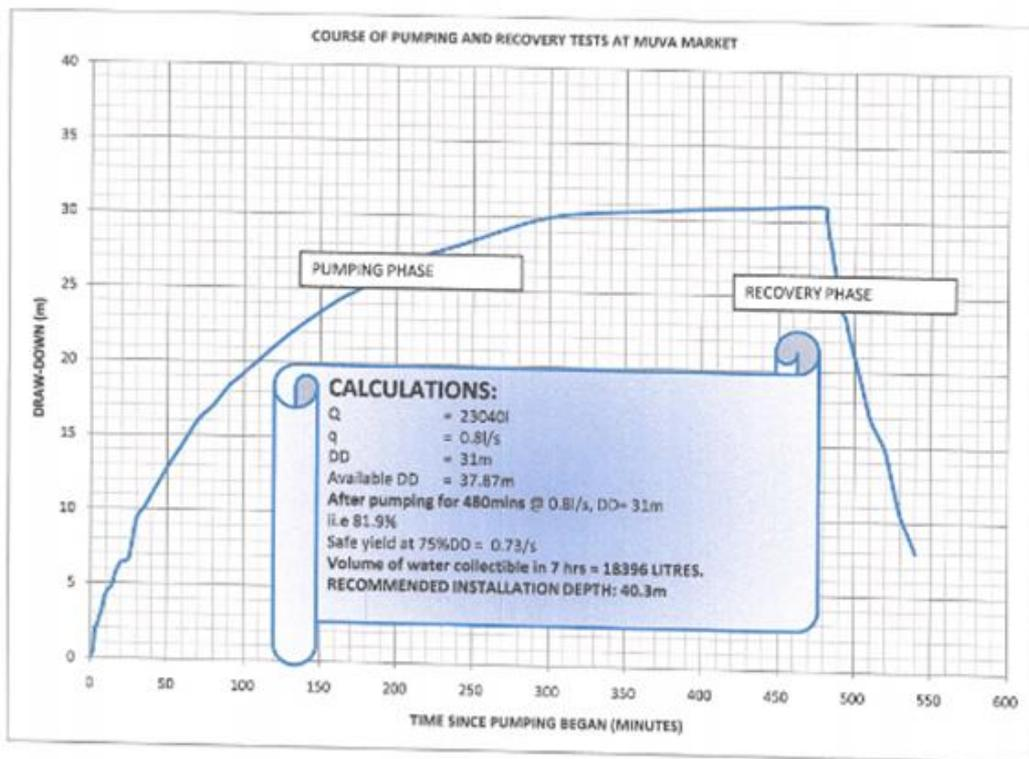
Fig. 4:Pumping and recovery curve for the recharging well
