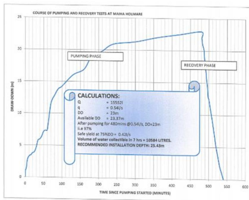
Fig. 6:Pumping and recovery curve for the recharging well
