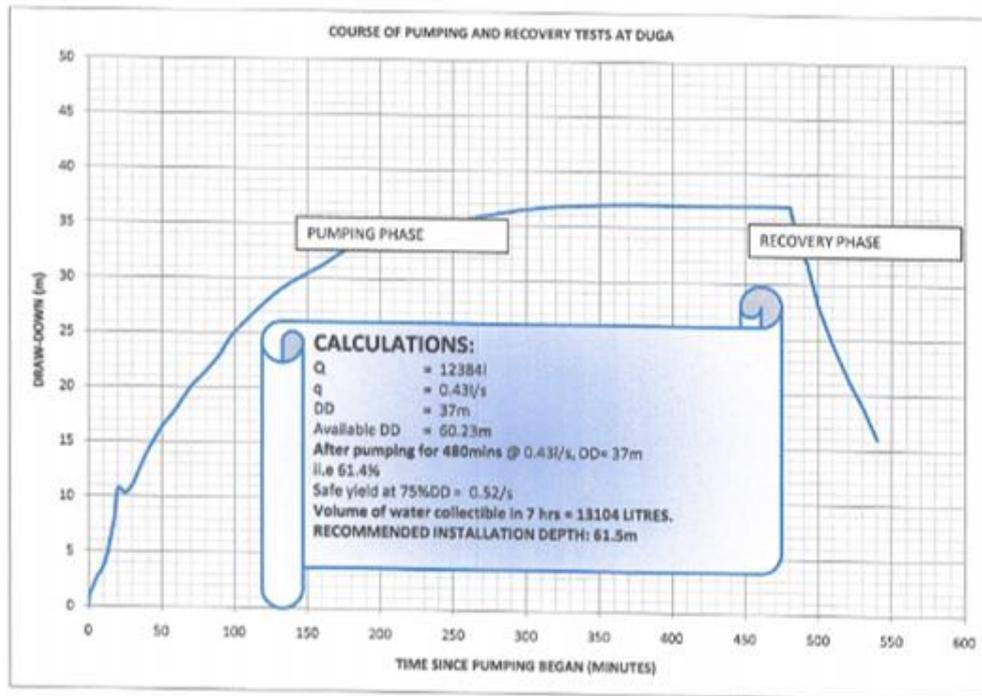
Fig. 5:Pumping and recovery curve for the recharging well
