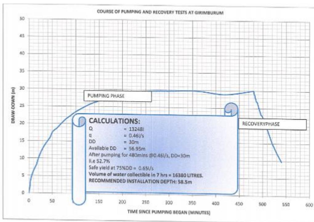
**Fig. 2:** Pumping and recovery curve for the recharging well
