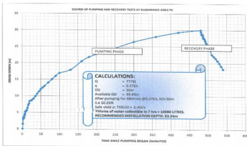
Fig. 3:Pumping and recovery curve for the recharging well
