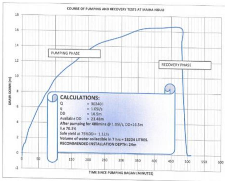
Fig. 7:Pumping and recovery curve for the recharging well
