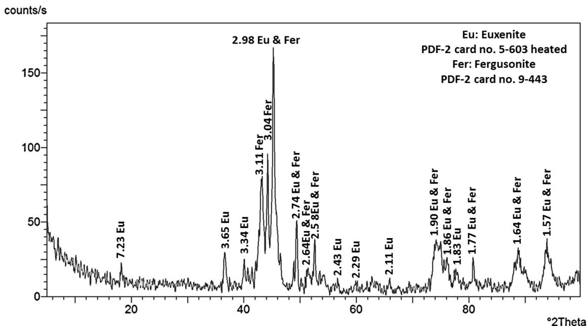
**Fig. 4:** XRD pattern for euxenite and fergusonite of Wadi El Sheih pegmatite sample
