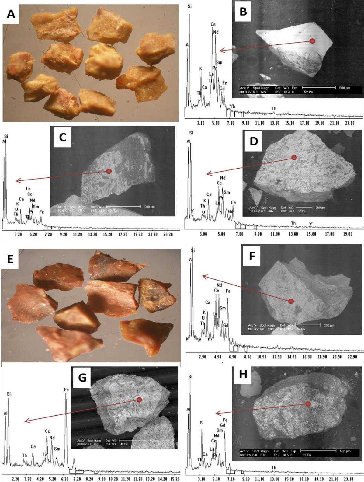
**Fig. 5:** Stereo microscopic images of yellowish brown allanite grains show the color and shape (A). BSE images and EDX spectrum of yellowish brown allanite grains show their chemical composition (B, C and D). Stereo microscopic images of reddish brown allanite grains show the color and shape (E). BSE images and EDX spectrum of yellowish brown allanite grains show their chemical composition (F, G and H).
