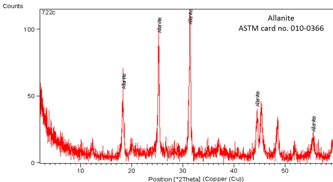
**Fig. 7:** XRD pattern for allanite of Wadi El Sheih pegmatite sample
