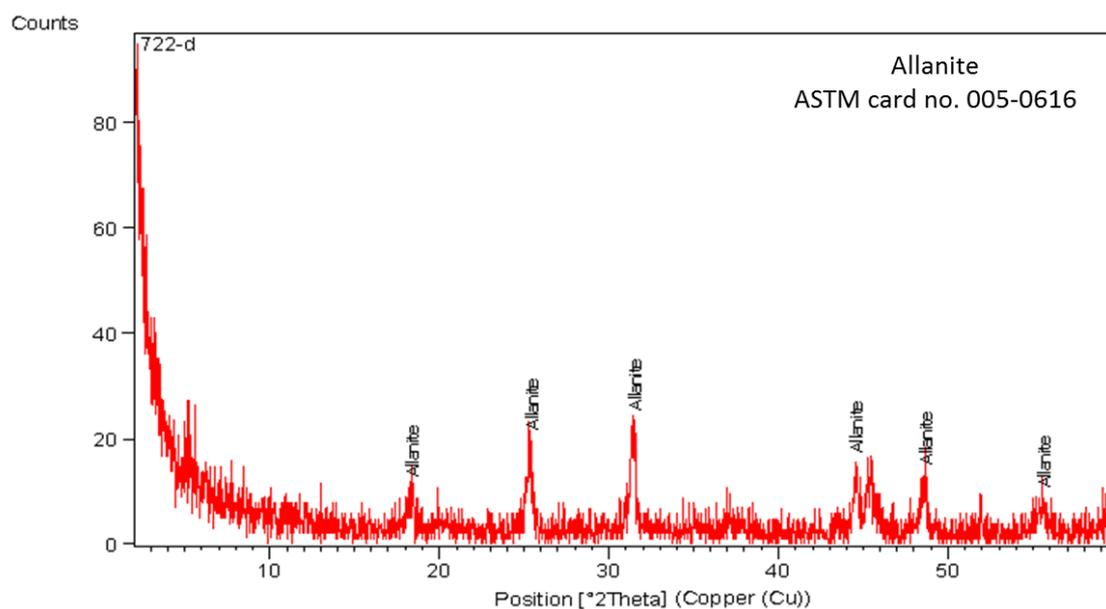
**Fig. 8:** XRD pattern for allanite of Wadi El Sheih pegmatite sample
