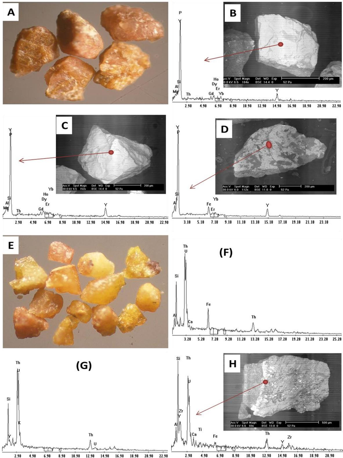
**Fig.9:** Stereo microscopic images of xenotime grains show the color and shape (A). BSE images and EDX spectrum of xenotime grains show their chemical composition (B, C and D). Stereo microscopic images of uranothorite grains show the color and shape (E). BSE images and EDX spectrum of uranothorite grains show their chemical composition (F, G and H)
