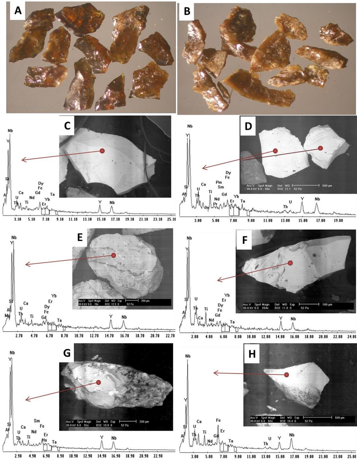
**Fig. 3:** Stereo microscopic images of fergusonite-Y grains show the color and shape (A&B). BSE images and EDX spectrum of fergusonite-Y grains show their chemical composition (C, D, E, F, G and H).
