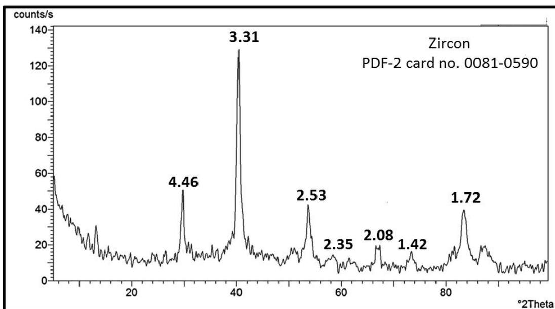
Fig.12: XRD pattern for Zircon of Wadi El Sheih pegmatite sample
