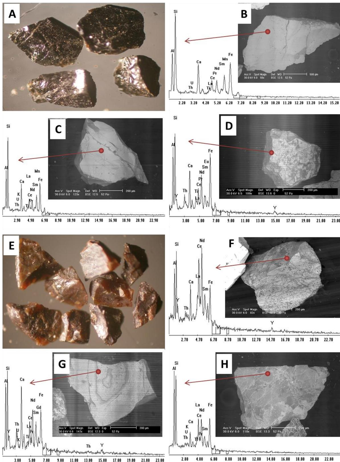
**Fig. 6:** Stereo microscopic images of black allanite grains show the color and shape (A). BSE images and EDX spectrum of black allanite grains show their chemical composition (B, C and D). Stereo microscopic images of dark brown allanite grains show the color and shape (E). BSE images and EDX spectrum of dark brown allanite grains show their chemical composition (F, G and H)
