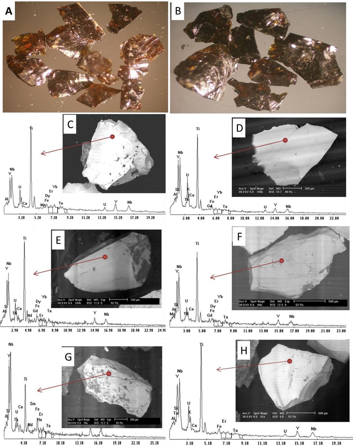
**Fig.2:** Stereo microscopic images of euxenite-Y grains show the color and shape (A-B). BSE images and EDX spectrum of euxenite-Y grains show their chemical composition (C, D, E, F, G and H).
