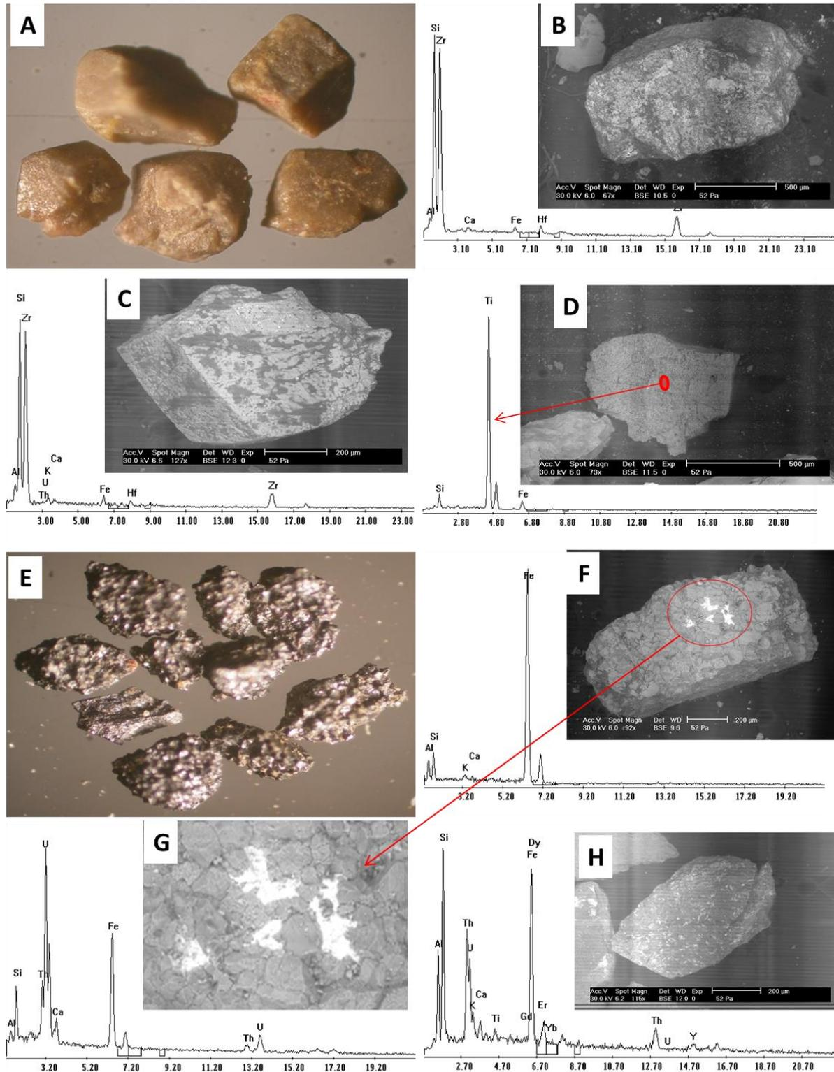
**Fig.10:** Stereo microscopic images of zircon grains show the color and shape (A). BSE images and EDX spectrum of zircon grains show their chemical composition (B, C and D). Stereo microscopic images of iron oxides grains show the color and shape (E). BSE images and EDX spectrum of iron oxides grains show their chemical composition (F, G and H)
