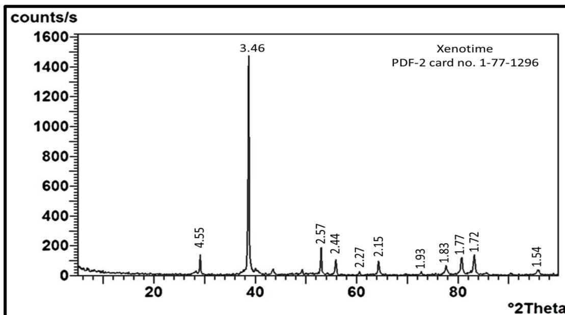
Fig.11: XRD pattern for xenotime of Wadi El Sheih pegmatite sample
