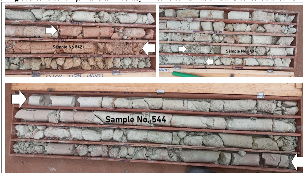
Figure 13: The depicted images illustrate the areas where samples 542, 543, and 544 were obtained from the COMM Borehole, and these sections consist solely of Smectite clays.
