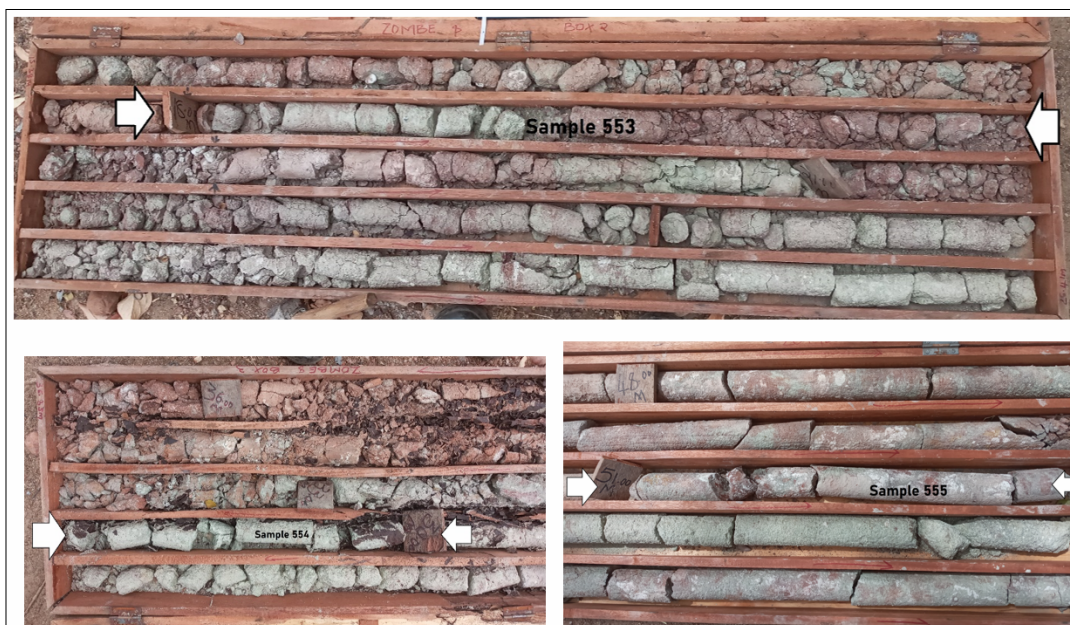
Figure 15: The depicted images illustrate the areas where samples 553, 554, and 555 were obtained from the COMM borehole, and these sections consist solely of nontronite clays.
