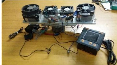
Fig:4 Experimental set up of thermoelectric generator with cooling fans and heat sink.
