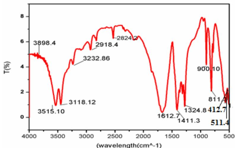
Figure 4: FTIR Spectrum of Oxalate-Ligand functional group assignments of NaCuOx crystal
