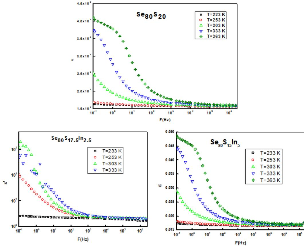
Fig [4] show the variation of dielectric constant ( $\epsilon'$ ) as a function frequency for the system  $Se_{80}S_{20-x}In_x$  where ( $x=0, 2.5, 5$ ).
