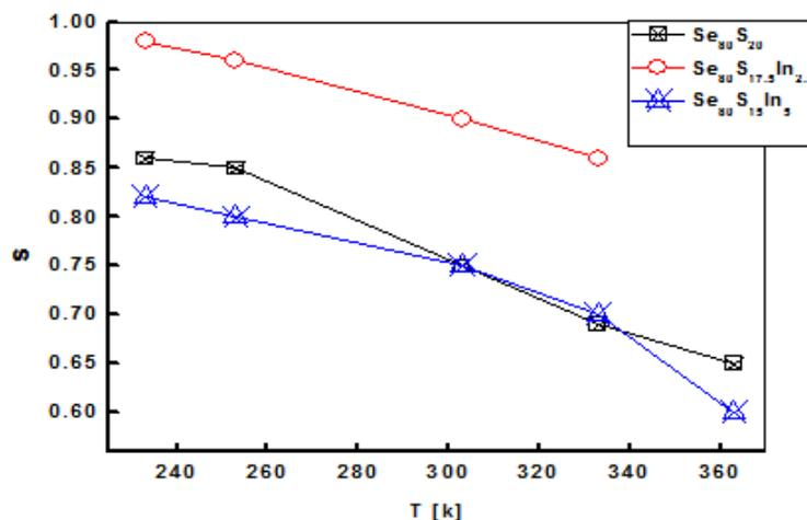
Fig [2] The exponent factor S as a function of temperature T of the system  $Se_{80}S_{20-x}In_x$  where  $(x=0,2.5,5)$ .
