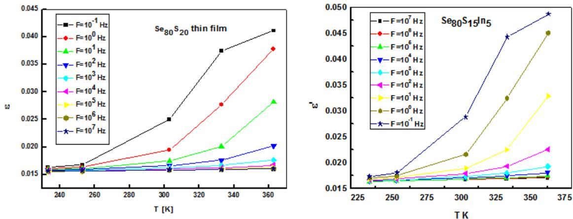
**Fig [6]** Variation of dielectric constant ( $\epsilon'$ ) as a function temperature at different frequency for the system  $Se_{80}S_{20-x}In_x$  where ( $x=0,2.5,5$ ).
