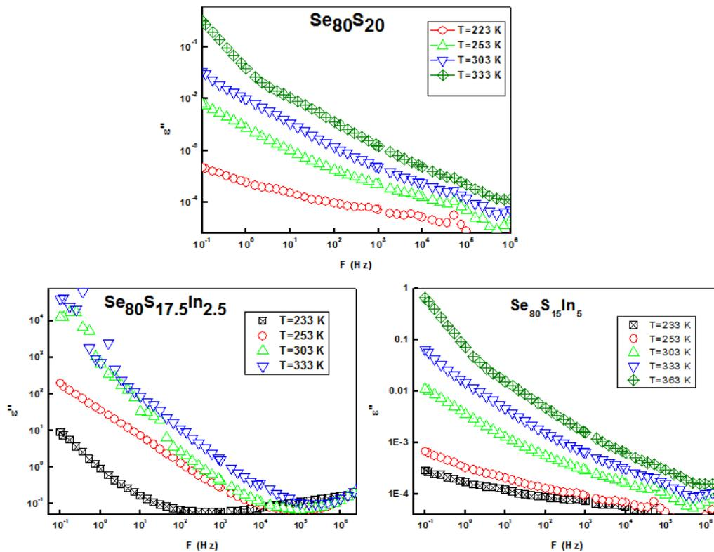
Fig [5] Variation of dielectric losses ( $\epsilon''$ ) as a function frequency at different isotherms for the system  $Se_{80}S_{20-x}In_x$  where ( $x=0, 2.5, 5$ ).
