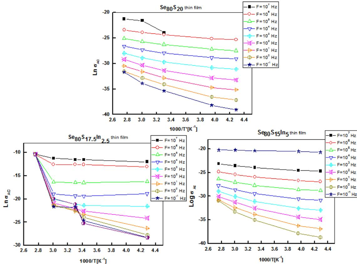
**Fig [3]** variation of  $\text{Ln } \sigma_{\text{Ac}}$  as a function  $1000/T$  at different constant frequency of the system  $\text{Se}_{80}\text{S}_{20-x}\text{In}_x$  where ( $x=0,2.5,5$ )
