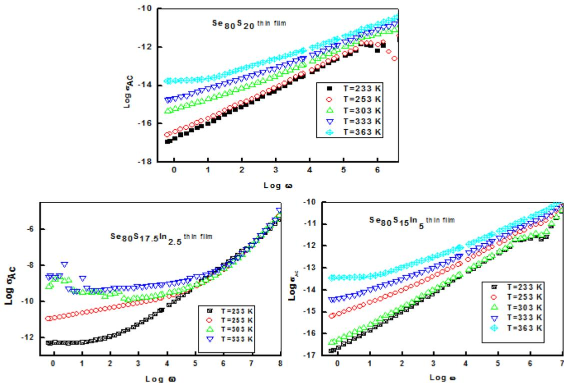
Fig [1] variation of  $\log \sigma_{Ac}$  as a function of  $\log \omega$  at different isotherms of the system  $Se_{80}S_{20-x}In_x$  where  $(x=0,2.5,5)$
