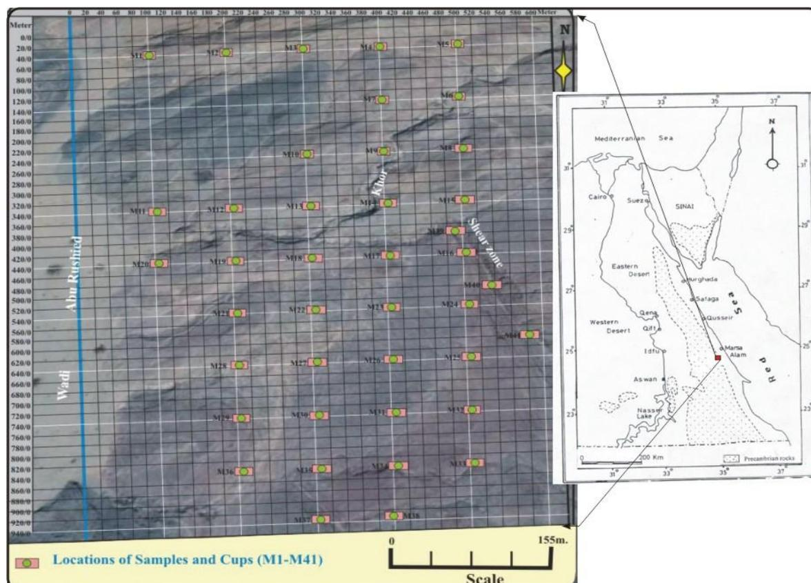
**Fig. (1):**Landsat map showing the location and net of samples in Abu Rushied area, South Eastern Desert.
