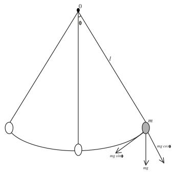
Figure 1: Simple Pendulum [8]
