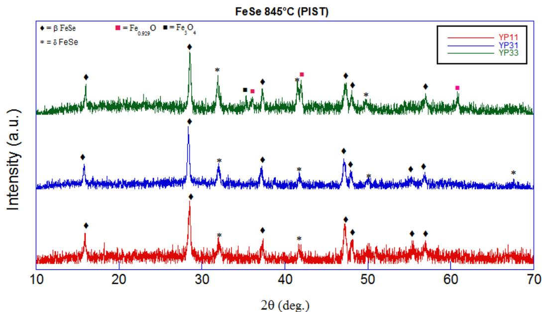
Figure 1. XRD Patterns of the KI Doped FeSe Sintered at 845°C for 3 h
