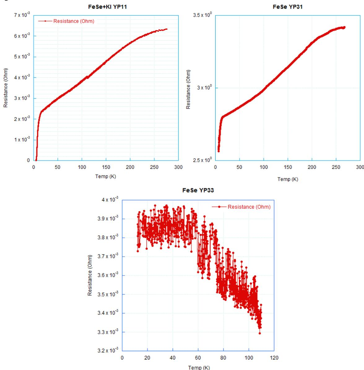
**Figure 2. Plot of Temperature vs Resistivity of the Mn Doped FeSe Samples**
