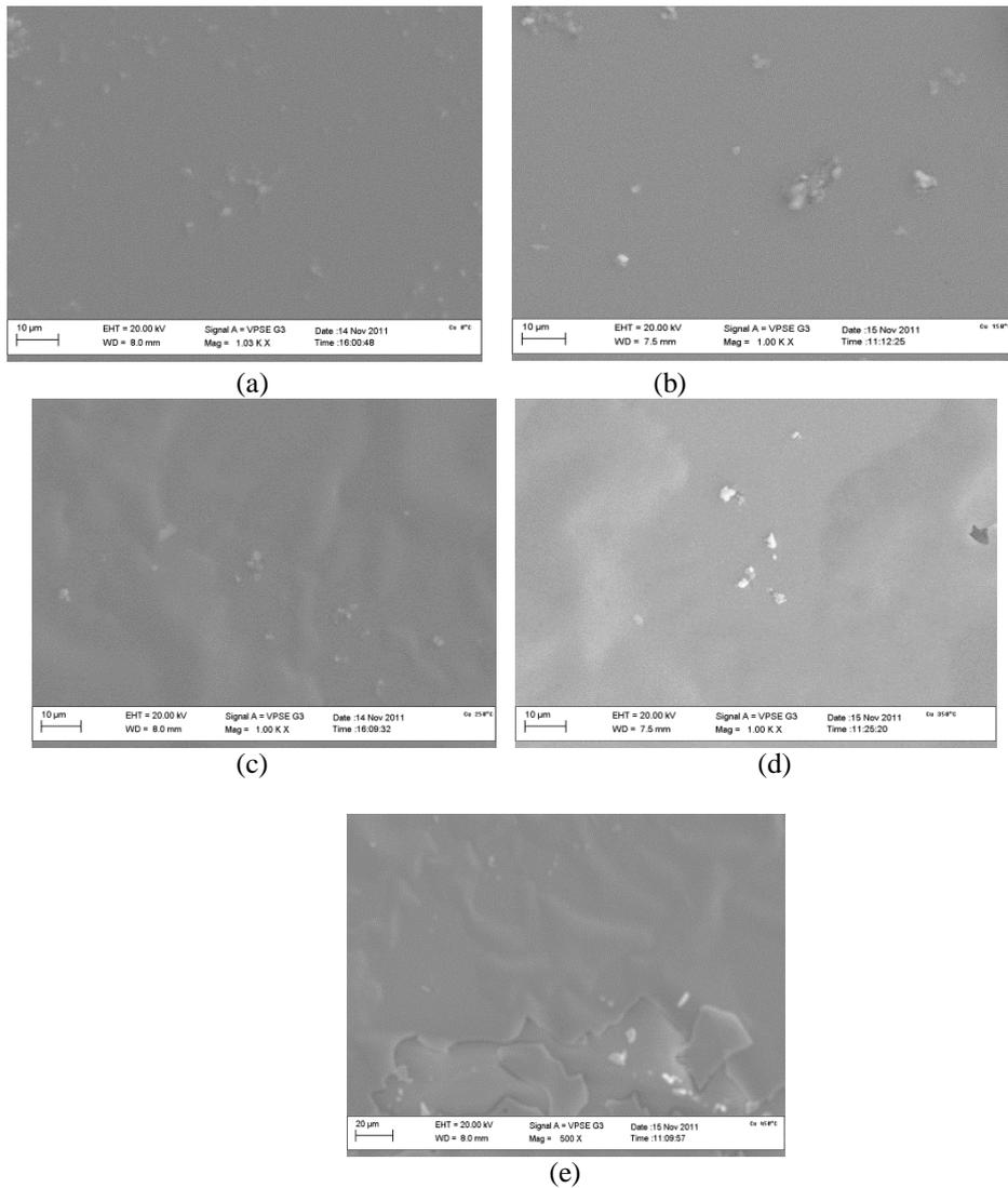
**Figure 3.** SEM image copper (a) as-deposited, (b) Cu film oxidized at 150 °C, (c) Cu film oxidized at 250 °C, (d) Cu film oxidized at 350 °C and (e) Cu film oxidized at 450 °C
