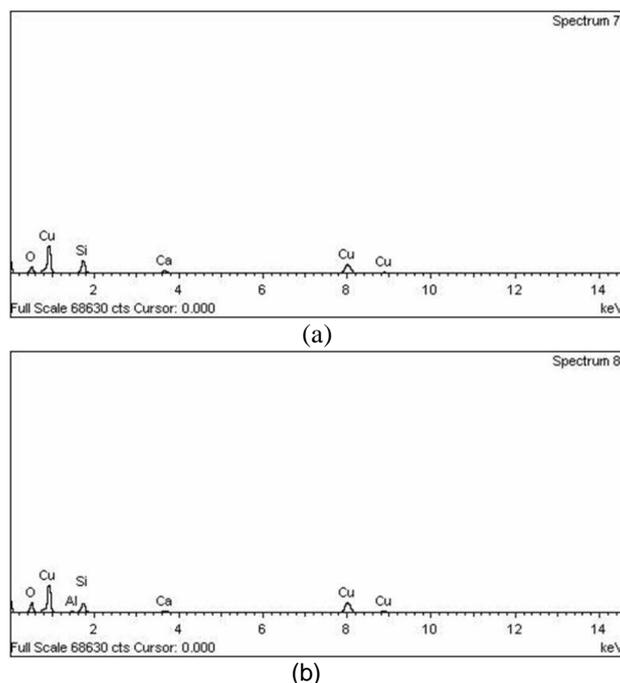
**Figure 2.** EDX spectrum of (a) Cu<sub>2</sub>O film and glass substrate (b) CuO and glass substrate
