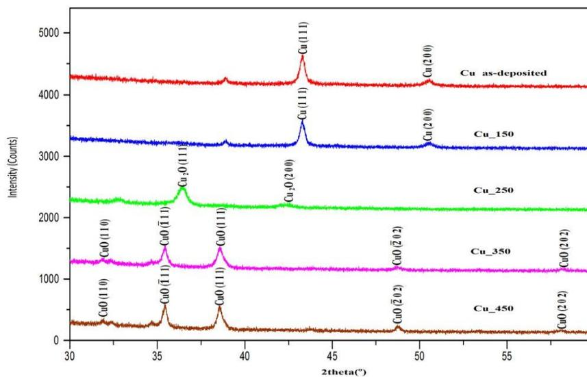
**Figure 1.** XRD pattern of Copper oxide films as a function of oxidation temperature
