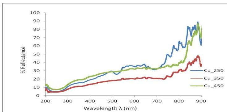
**Figure 4.** Reflectance spectra of Copper oxide films oxidised at 250, 350 and 450 °C
