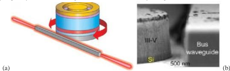
Fig(18): (a) Hybrid micro-ring laser with a Si bus waveguide. (b)SEM image of resonator sidewall and bus waveguide
