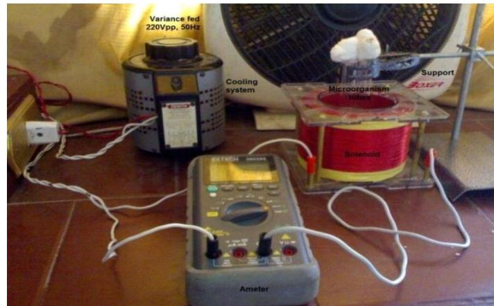
Fig. (1a): The electromagnetic field exposure system.
