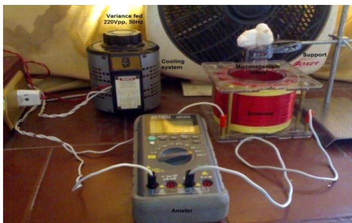
Fig. (1a): The electromagnetic field exposure system.
