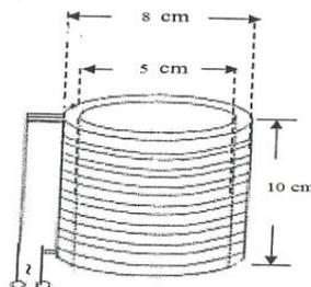
Fig. (1b): A diagram of the solenoid characteristics.
