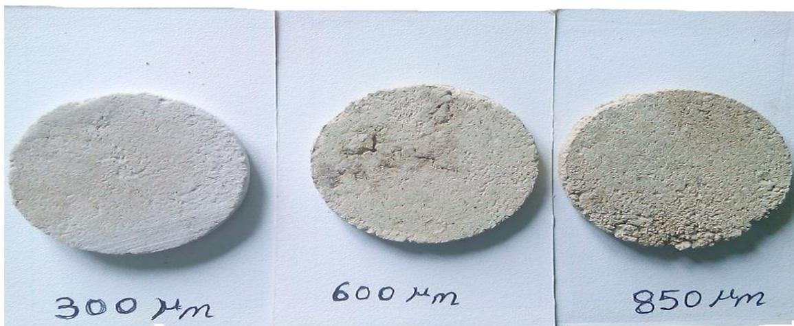
**Figure 1:** Final disc shape of the samples for different particle sizes
