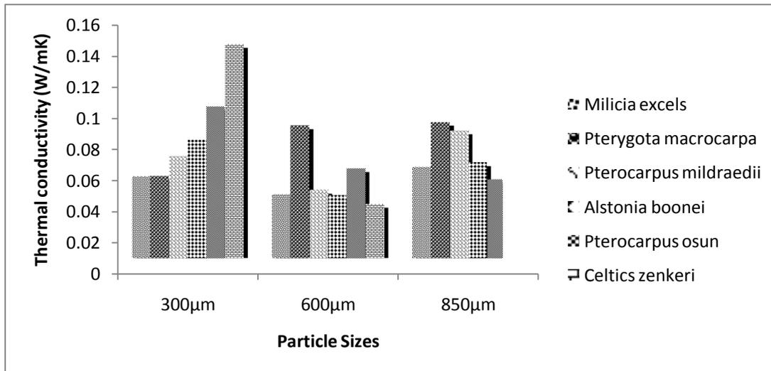
Figure 2: Thermal conductivities of samples at 300, 600 and 850 µm particle sizes
