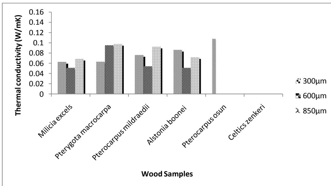
Figure 3: Thermal Conductivities of different particle sizes for each wood sample
