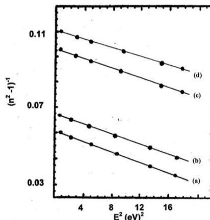
Figure.8 – Variation of  $(n^2 - 1)^{-1}$  versus (Photon Energy)<sup>2</sup> for ZnS films deposited at different duty cycles (a) 50 % (b) 33 % (c) 15 % (d) 6 %
