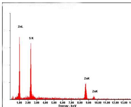
Figure.2 – EDS spectrum of ZnS films deposited at 50 % duty cycle
