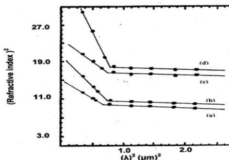
Figure.7 – Variation of (refractive index)<sup>2</sup> with (wavelength)<sup>2</sup> of ZnS films deposited at different duty cycles (a) 6 % (b) 15 % (c) 33 % (d) 50 %
