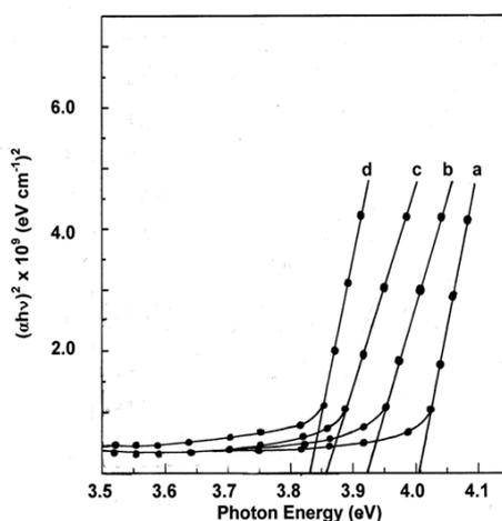
Figure.5 – Tauc’s plot of ZnS films deposited at different duty cycles (a)50 % (b) 33 % (c) 15 % (d) 6 %
