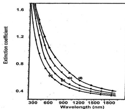
Figure.6 - Variation of extinction co-efficient with wavelength of ZnS films deposited at different duty cycles (a) 6 % (b) 15 % (c) 33 % (d) 50 %
