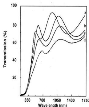
Figure.3 – Transmission spectra of ZnS films deposited at different duty cycles (a)50% (b) 33% (c) 15% (d) 6 %
