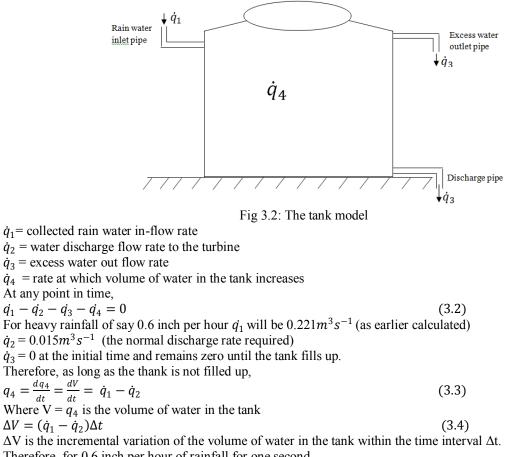
Therefore, for 0.6 inch per hour of rainfall for one second  $\Delta V = (0.0221 \text{m}^3 \text{s}^{-1} - 0.015 \text{m}^3 \text{s}^{-1}) (1\text{s})$
