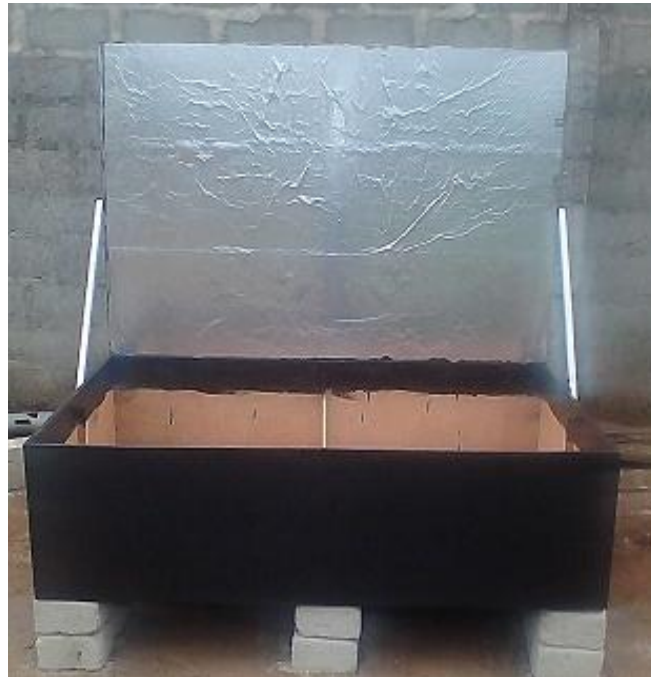
Fig. 2.1 The constructed outer box with reflector
