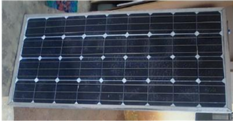
Fig. 3.4 The constructed solar panel
