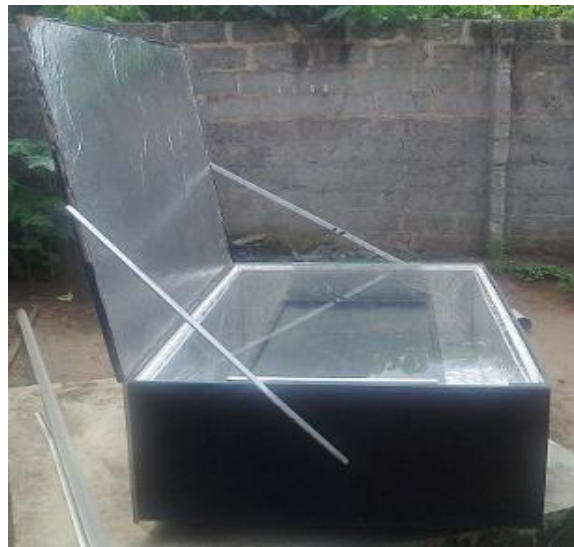
Fig. 2.3 The one reflector solar oven for solar panel lamination
