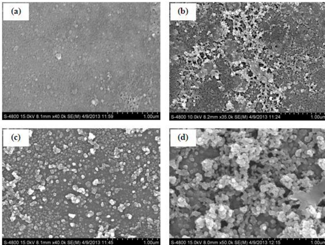
**Fig. 3** Surface Morphology of  $\text{Ag}_2\text{S}$  thin film synthesized with: a) 20, b) 30, c) 40 and d) 50 immersion cycles.
