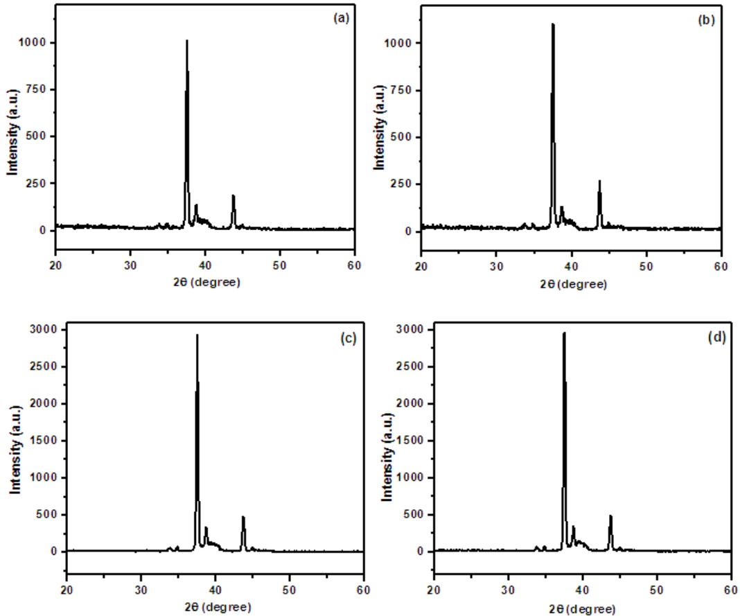
**Fig. 2** XRD pattern of Ag<sub>2</sub>S thin film synthesized with: a) 20, b) 30, c) 40 and d) 50 immersion cycles.
