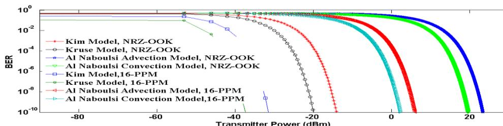
Fig. (15) BER versus Transmitter Power for 950 nm, V=1km, L=1km.
