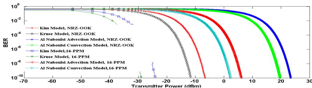
Fig. (14) BER versus Transmitter Power for 850 nm, V=1km, L=1km.
