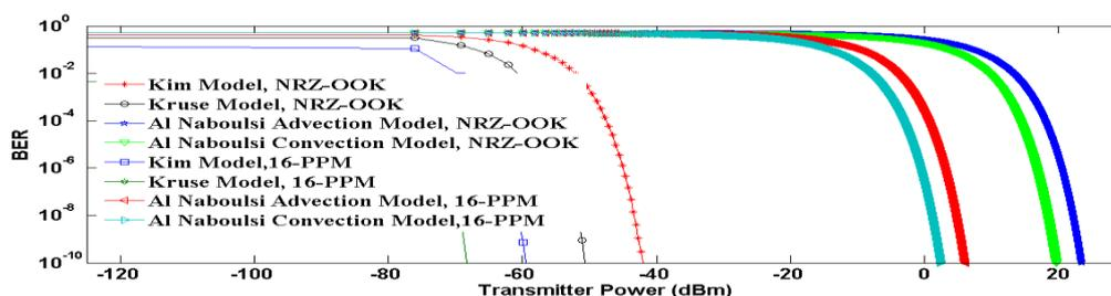
Fig. (16) BER versus Transmitter Power for 1550 nm, V=1km, L=1km.
