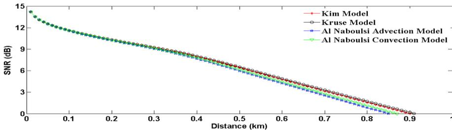
Fig (5) SNR for 650 nm
