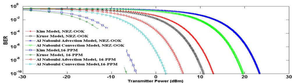
Fig. (13) BER versus Transmitter Power for 650 nm, V=1km, L=1km.
