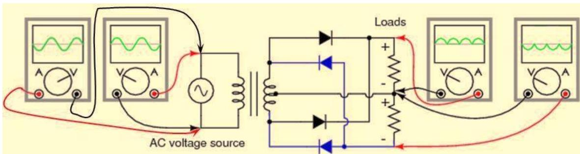
**Fig. 2.6.8i** Full wave rectifier (secondary voltage = V/2)
