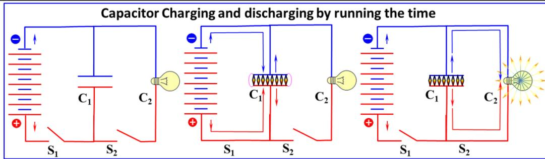
**Fig.2.10c** Capacitor charging and discharging by running the time
