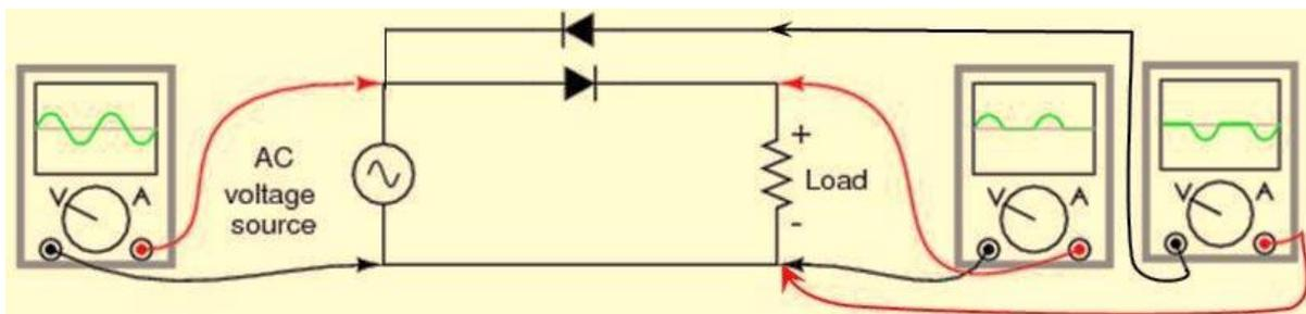
**Fig. 2.6.8h** Half wave rectifier, (4 nos of half cycle AC wave form =4nos of half cycle DC waveform)
