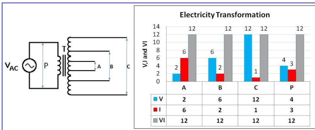
**Fig. 2.6a** Characteristic Properties of Power Transformer ( $VI=C$ ) in 2D graph
