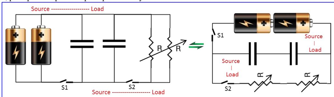
**Fig. 2.4.1** Combinations of Capacitor with load under conversion process (charging and discharging)
