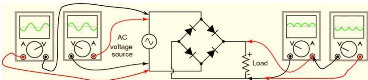
**Fig 2.6.8j** Bridge Rectifier (secondary utilized voltage = V)
