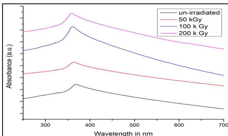
**Figure 2:** UV-Vis spectroscopic analysis of un-irradiated and irradiated ZnO nanoparticles
