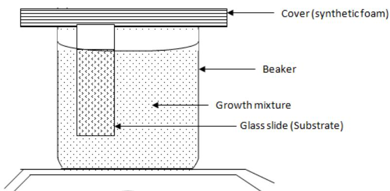
Fig. 1. Experimental set up.
