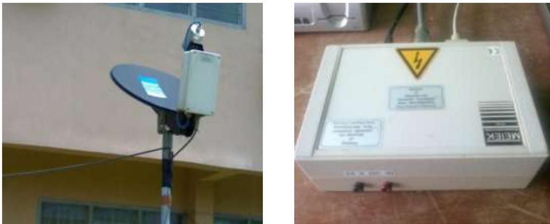
Figure 2: Experimental set up showing (a) the outdoor unit and (b) indoor unit of the MRR.
