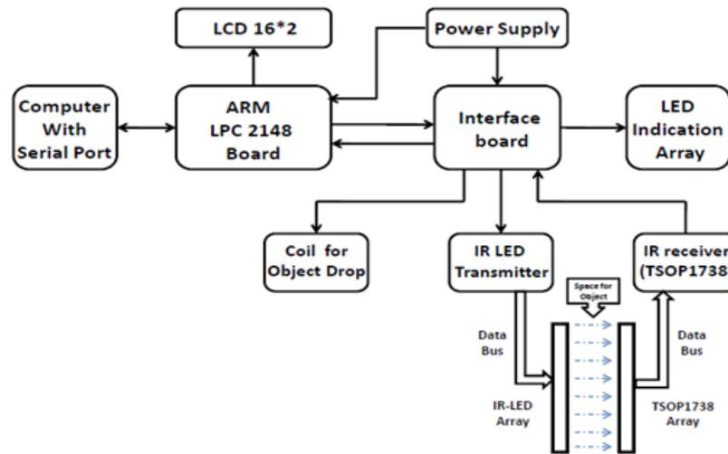
Fig.1 Block diagram of event counter circuit.
