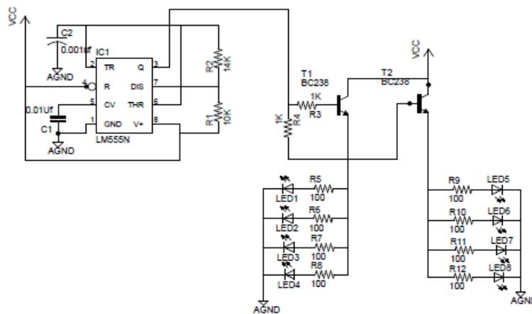
Figure 2. Astable multivibrator with 1 IR Transmitters
