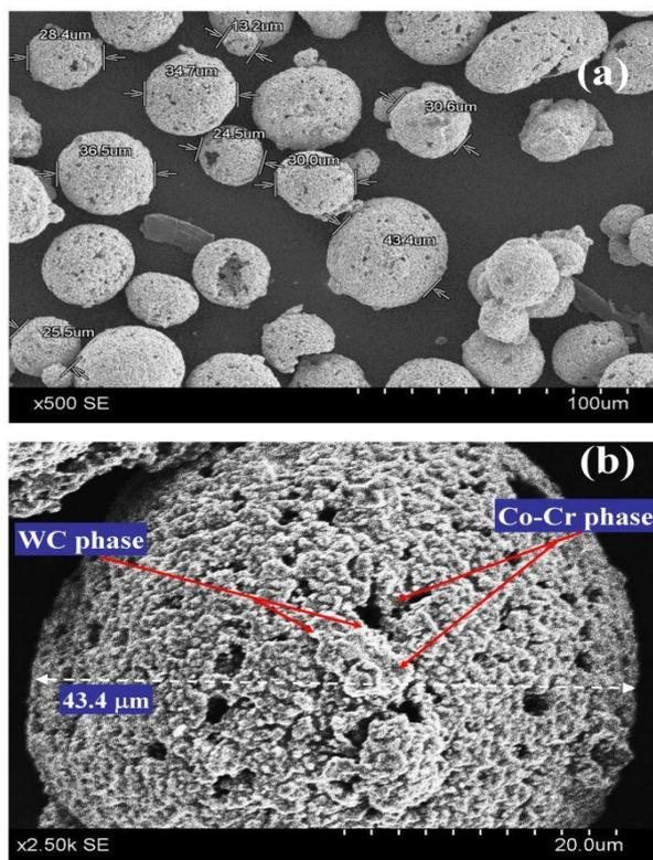
Figure 1. SEM picture of WC-CoCr (a) powders (b) a single particle
