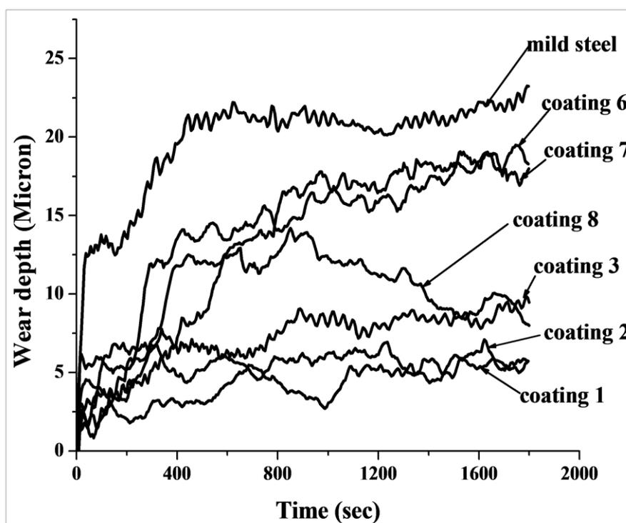
Figure 5. Wear depth Vs time plot for coated and uncoated specimens
