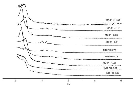
**Fig. 2:** XRD Patterns of SBA16 at different pH of synthesis gel. The FT-IR spectra of as synthesized SBA16 from Rice husk ash:
