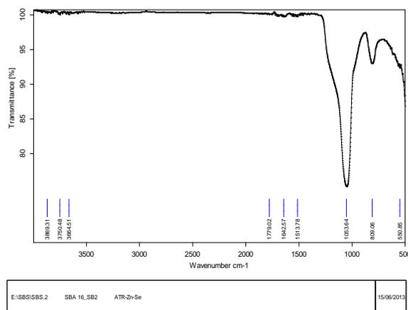
**Figure 3:** The FT-IR Spectra Of As Synthesized SBA16 From Rice Husk Ash Antibacterial Activity Of  $\text{TiO}_2$ -Containing SBA-16:
