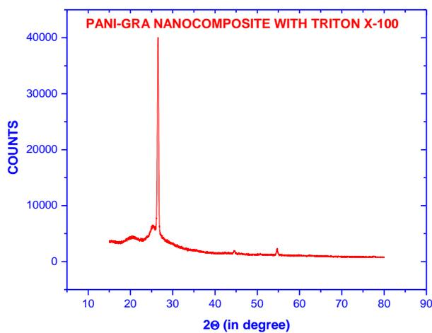
Fig.5: XRD of PANI-GRA nanocomposite treated with triton x-100.
