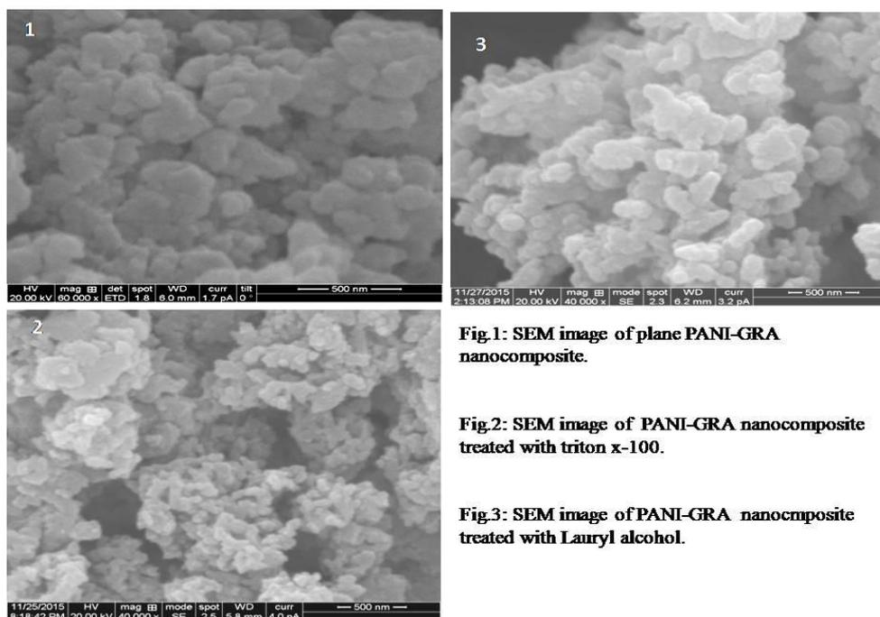
**Fig.1: SEM image of plane PANI-GRA nanocomposite.**
