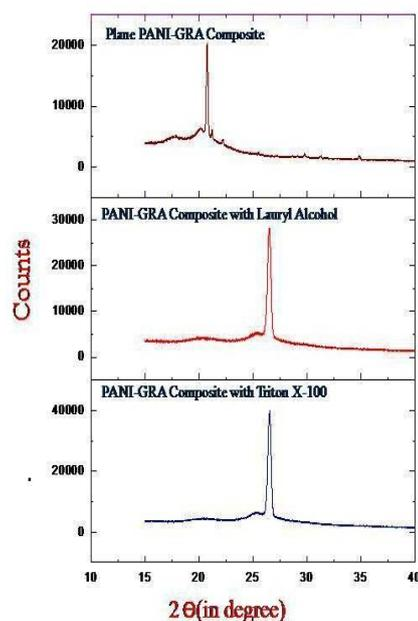
Fig. 6: Combined XRD of three nanocomposites shows peak shift towards higher value of  $2\theta$
