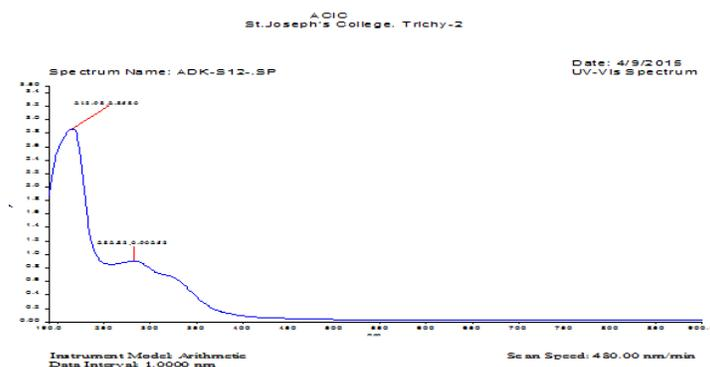
**Fig.2-UV-Visible spectrum of synthesized silver nanoparticles using leaf extracts of Ipomoea staphylina.**
