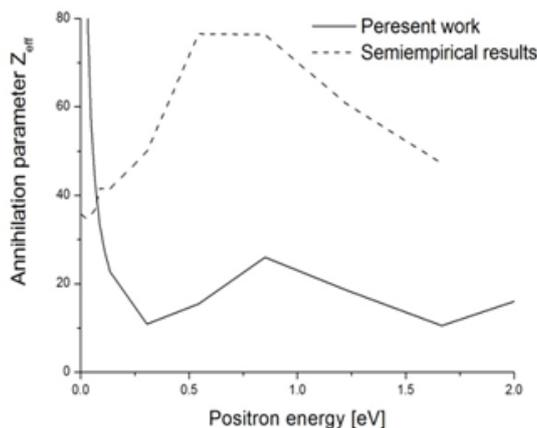
**Fig. 3:** The energy dependence of annihilation parameters  $Z_{\text{eff}}$  of positron. The solid line is the present results. The dashed lines are the semi-empirical results calculated by Mitroy and Ivanove [27].
