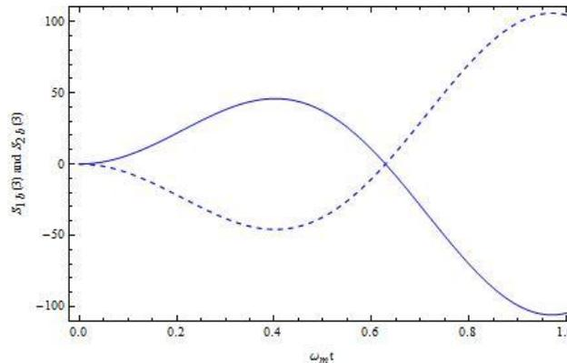
**Figure 2:** Plot of squeezing parameter  $S_{1b}(3)$  and  $S_{2b}(3)$  with  $\omega_m t$  for  $b$  mode with  $n=3$ ,  $\alpha = 3$ ,  $\beta = 2$ ,  $g = 2\pi \times 10$  KHz and  $\frac{g}{\omega_m} = 0.1$
