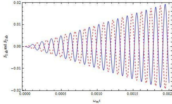
**Figure 4:** Plot of squeezing parameter  $S_{1ab}$  and  $S_{2ab}$  with  $\omega_m t$  for  $ab$  compound mode with  $\alpha = 3$ ,  $g = 2\pi \times 10$  KHz and  $\frac{g}{\omega_m} = 0.1$ .
