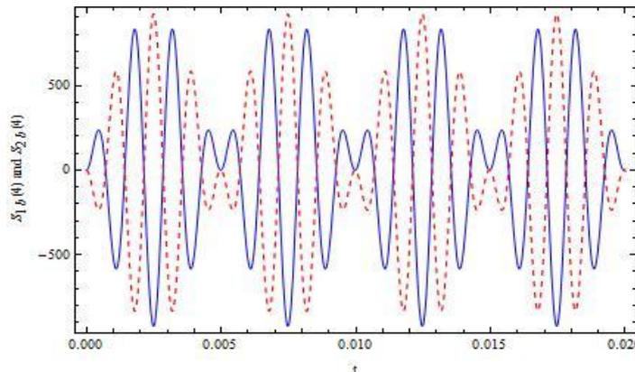
**Figure 2:** Plot of squeezing parameter  $S_{1b}(4)$  and  $S_{2b}(4)$  with  $t$  (ms) for  $b$  mode with  $n=4$ ,  $\alpha = 3$ ,  $\beta = 2$ ,  $g = 2\pi \times 10$  KHz and  $\frac{g}{\omega_m} = 0.1$ .
