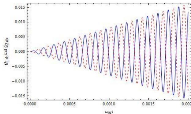
**Figure 5:** Plot of squeezing parameter  $Q_{1ab}$  and  $Q_{2ab}$  with  $\omega_m t$  for  $ab$  compound mode with  $\alpha = 3$ ,  $g = 2\pi \times 10$  KHz and  $\frac{g}{\omega_m} = 0.1$ .
