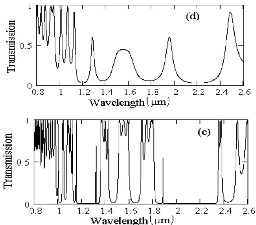
**Figure 1** Calculated transmission coefficient vs wavelength for symmetrical Fibonacci ZnS/MgF<sub>2</sub> multilayers with different generations. SFM S<sub>5</sub> with 16 layers (a) with symmetry, (b) without symmetry; SFM S<sub>6</sub> with 26 layers (c) with symmetry, (d) without symmetry; SFM S<sub>8</sub> with 68 layers (e) with symmetry.
