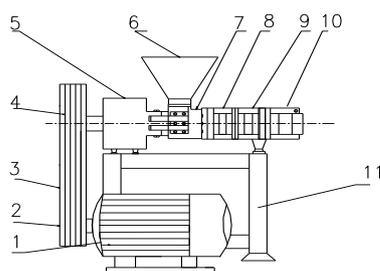
1. Motor 2. Small pulleys 3. Belt 4. Large pulleys 5. bearing block 6. feed hopper 7. Barrel piece 1<sup>st</sup> 8. Barrel piece 2<sup>nd</sup> 9. Barrel piece 3<sup>rd</sup> 10. Barrel piece 4<sup>th</sup> 11. Rack
