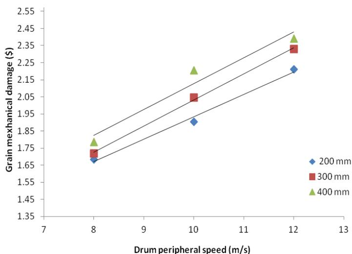
**Fig. 6** Grain damage versus peripheral drum speed at different levels of drum diameter
