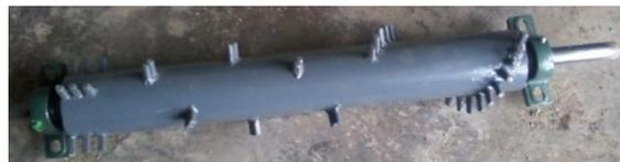
**Fig. 2:** *Threshing drum and concave*
