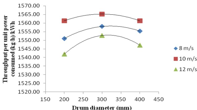
Fig.7: Effect of drum speed on throughput per unit power consumption
