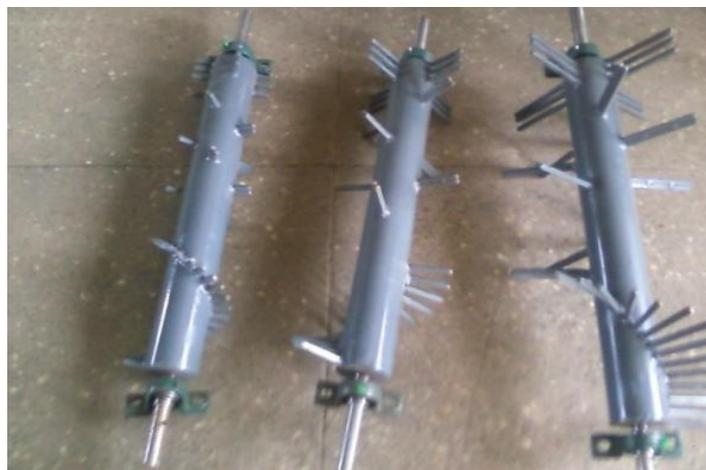
**Fig. 3:** Threshing drums of different diameters
