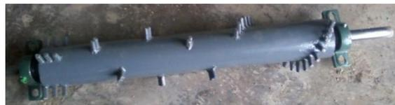
**Fig. 2:** *Threshing drum and concave*
