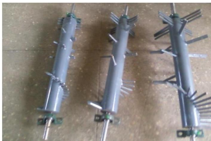
**Fig. 3:** Threshing drums of different diameters
