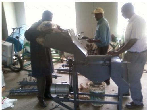
Fig 4: Threshing operation using the prototype thresher
