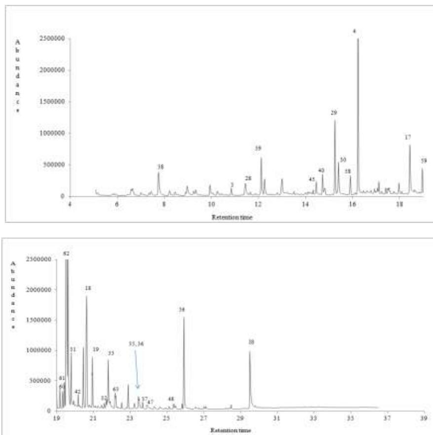
**Figure 3.** A typical chromatogram of commercial thyme honey from New Zealand. Possible volatile markers are numbered according to Table 3. IS: internal standard (benzophenone).
