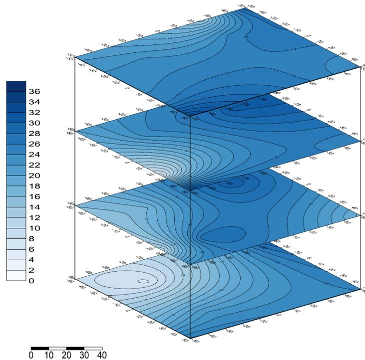
**Fig.1: Soil moisture patterns under mini-sprinkler**
