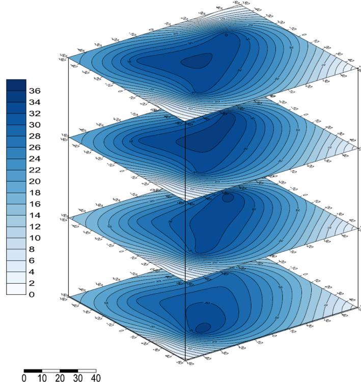
**Fig.2: Soil moisture patterns under drip**
