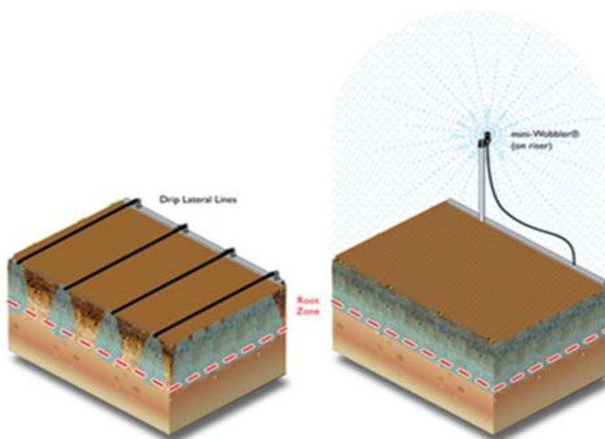
**Fig.3:** The performance of mini-sprinkler and drip on soil moisture distributions.
